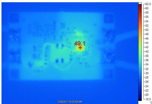
Figure 12. Thermal Image at  $V_{IN} = 36$  V
