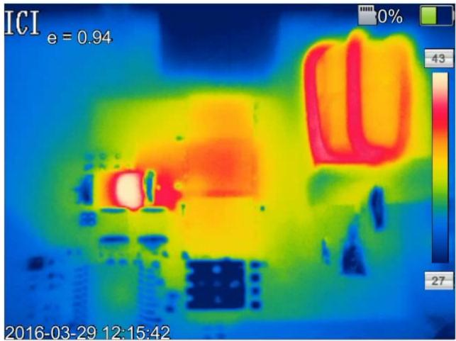
Vin =12V; Iout=12A (max temp 43C)
