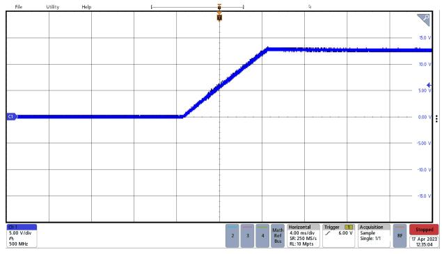
Figure 3-1. PMP20634C Output Voltage Start-Up
