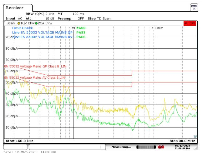
Figure 3-8. Measurement With 120-VAC, 60-Hz Input, Line Neutral Flipped
