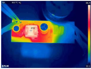
Figure 2-3. Thermal Image, 120-VAC, 60-Hz Top
