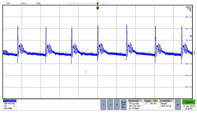
Figure 3-2. Output Voltage Ripple 12-V, 1-A
