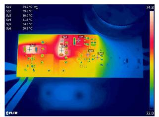
Figure 2-4. Thermal Image, 230-VAC, 50-Hz Bottom
