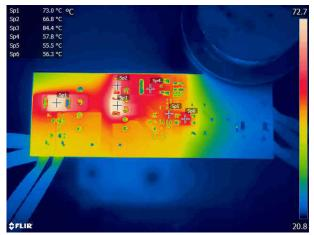
Figure 2-2. Thermal Image, 120-VAC, 60-Hz Bottom
