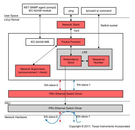
Figure 11. PRU-ICSS Enabled Fast Cut-Through Switch
