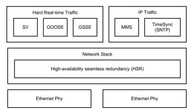
Figure 1. System Architecture
