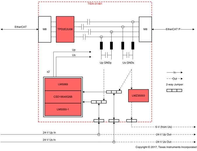
Figure 1. Block Diagram of TIDA-01461
