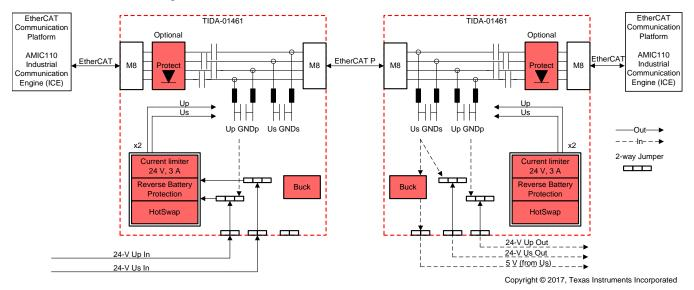
Figure 2. System Block Diagram With Two AMIC110 ICEs and Two TIDA-01461 Boards
