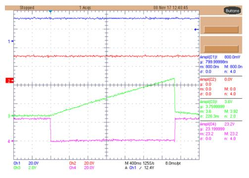
Figure 13. Short-Circuit Behavior—V<sub>in</sub> (1), GQ1 (2), C<sub>timer</sub> (3), V<sub>out</sub> (4)
