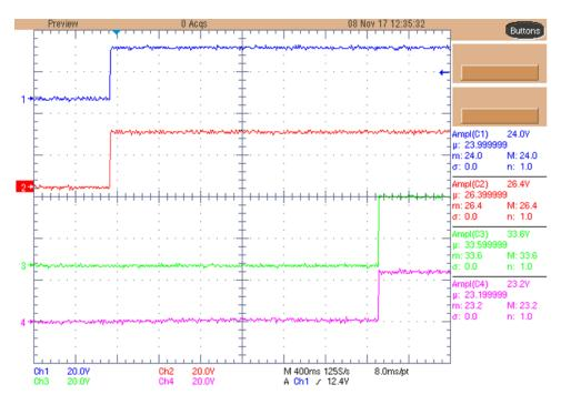
Figure 10. Power-up Sequence—V<sub>in</sub> (1), GQ1 (2), GQ2 (3), V<sub>out</sub> (4)
