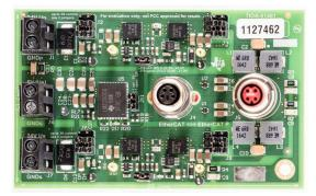
EtherCAT P®—One Cable for Power and EtherCAT® Reference Design
