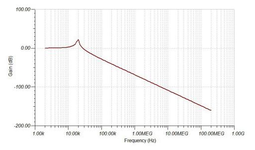
Figure 7. Bode Plot of Second-Order LC Low-Pass Filter (L = 6.8  $\mu$ H and C = 10  $\mu$ F)
