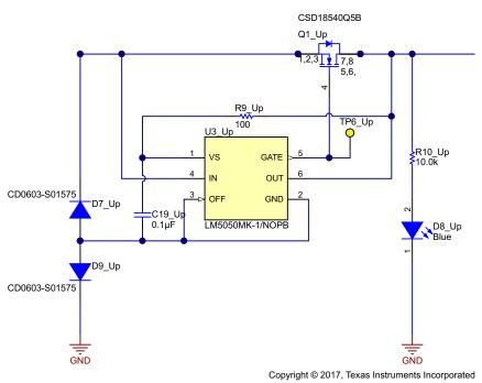
Figure 3. Schematic of Reverse Polarity Protection With LM5050-1
