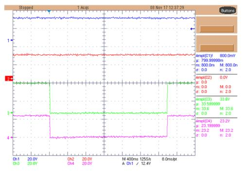
Figure 12. Short-Circuit Behavior—V<sub>in</sub> (1), GQ1 (2), GQ2 (3), V<sub>out</sub> (4)
