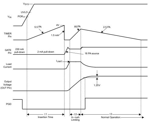
Figure 5. Power-up Sequence (Current Limit Only) of LM5069
