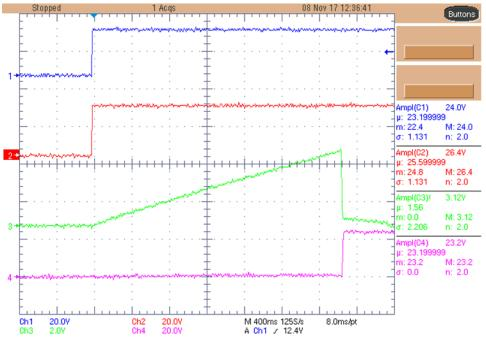
Figure 11. Power-up Sequence— $V_{in}$  (1), GQ1 (2), C<sub>timer</sub> (3), V<sub>out</sub> (4)
