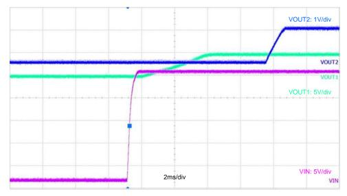
Figure 13. Start-Up Waveform:  $V_{IN} = 24 V$ ,  $I_{OUT2} = 0 A$
