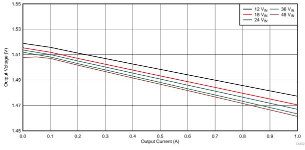
Figure 12. TPS62821 Load Regulation: Vout2 vs Iout2
