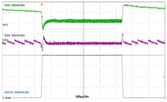
Figure 17. Load Transient:  $V_{IN}$  = 24 V,  $I_{OUT1}$  = 0 A,  $I_{OUT2}$  = 0 A to 1 A to 0 A,  $t_R$  =  $t_F$  = 10 µs
