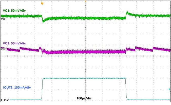
Figure 19. Load Transient:  $V_{IN}$  = 24 V,  $I_{OUT1}$  = 300 mA,  $I_{OUT2}$  = 0 A to 300 mA to 0 A,  $t_R$  =  $t_F$  = 10 µs
