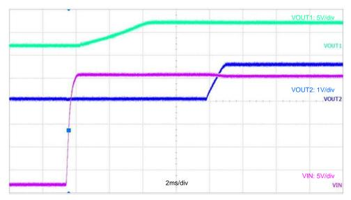
Figure 14. Start-Up Waveform:  $V_{IN} = 24 V$ ,  $I_{OUT2} = 1 A$
