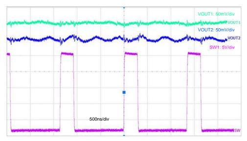
Figure 16. Steady-State Waveform:  $V_{IN} = 24 V$ ,  $I_{OUT2} = 1 A$
