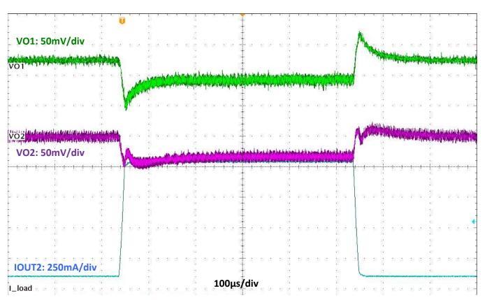
Figure 18. Load Transient:  $V_{IN}$  = 24 V,  $I_{OUT1}$  = 300 mA,  $I_{OUT2}$  = 0.1 A to 1 A to 0.1 A,  $t_R$  =  $t_F$  = 10 µs
