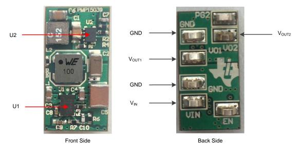
Figure 6. PMP15039 Board Setup
