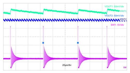
Figure 15. Steady-State Waveform:  $V_{IN} = 24 \text{ V}, I_{OUT2} = 10 \text{ mA}$
