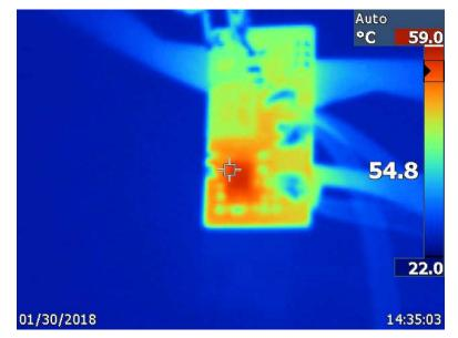
Figure 8. PMP15039 Thermal Image:  $V_{IN}$  = 24 V,  $I_{OUT1}$  = 300 mA,  $I_{OUT2}$  = 1 A
