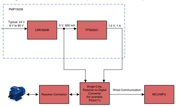
Figure 2. PMP15039 for AC Drive Position Feedback Applications
