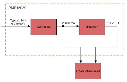
Figure 3. PMP15039 Block Diagram
