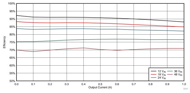
Figure 10. System Efficiency Versus Load Current:  $I_{OUT1} = 0.3 A$ ,  $I_{OUT2} = 0 A$  to 1 A
