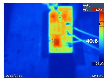
Figure 7. PMP15039 Thermal Image:  $V_{IN} = 24 V$ ,  $I_{OUT1} = 0 A$ ,  $I_{OUT2} = 1 A$
