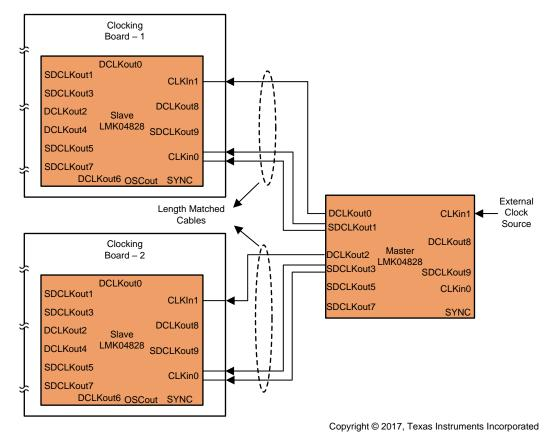
Figure 2. Tree Configuration of Multiple LMK04828 Devices
