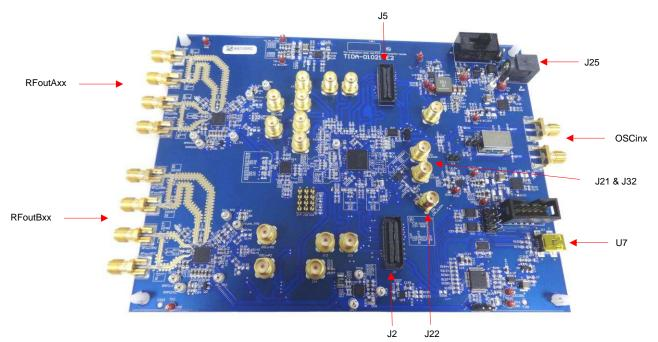
Figure 6. Multichannel Clocking Board Hardware
