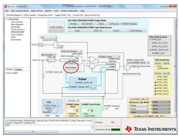
Figure 9. TICSPro-SW GUI for Send Pulses
