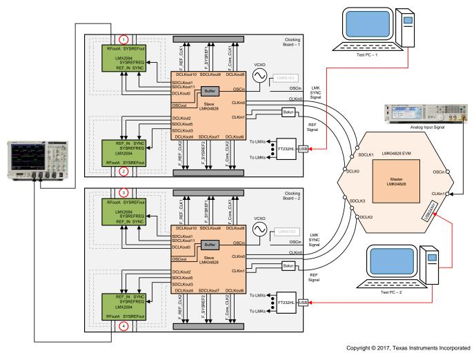
Figure 11. Test Setup for Multiboard Clock Skew Measurement
