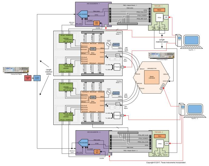
Figure 12. Test Setup for ADC12DJ3200 SNR and Channel-to-Channel Skew Measurement
