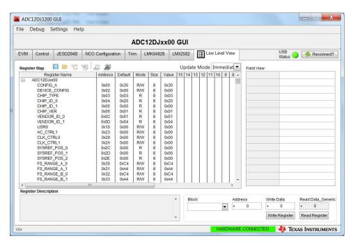
Figure 7. ADC12DJ3200 EVM Programming
