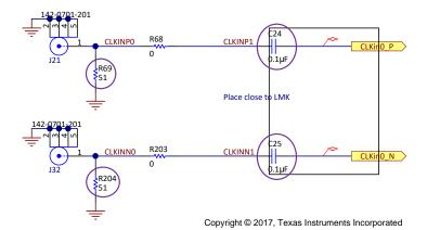
Figure 3. Clocking Board 2—LMK04828 CLKin0 Path Modification for DC-Coupled SYNC Inputs
