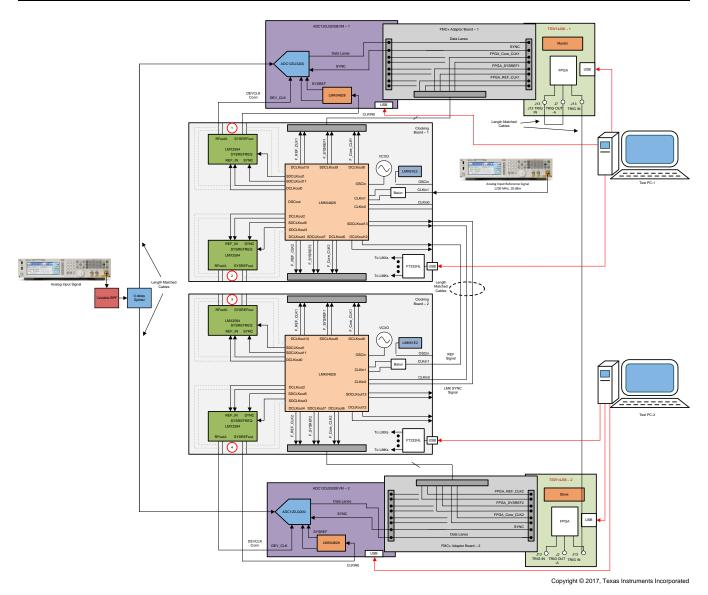
Figure 9. Test Setup for ADC12DJ3200 SNR and Channel-to-Channel Skew Measurement
