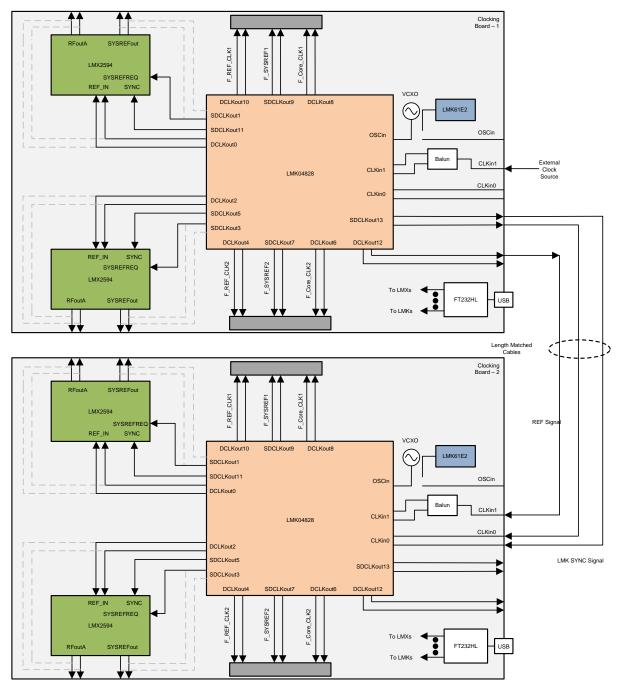
Figure 1. Daisy-Chain Configuration for Synchronizing Multiple Clocking Boards
