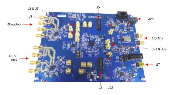
Figure 5. Multichannel Clocking Board Hardware
