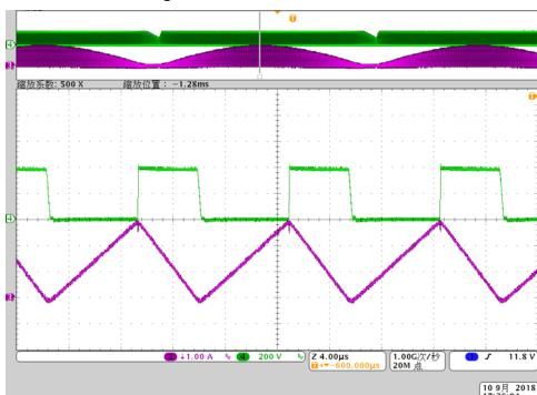
Figure 8. PFC-115 VAC at Full-load
