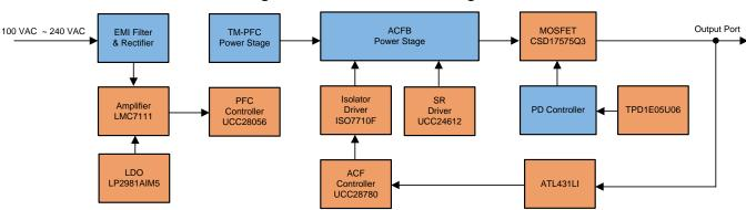
Figure 1. TIDA-01623 Block Diagram
