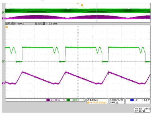
Figure 10. SW-PFC-230 VAC at Full-load
