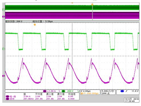
Figure 13. SW-ACF-115 VAC, 20 V<sub>out</sub>, 3.75 A
