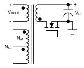
The Na1 winding is designed to power the devices at 5-V and 9-V outputs. Considering the voltage derating at a light load, there should be enough margin on VDD\_min. Then at a 9-V output, the VDD is equal to the TVS diode voltage of 16 V. Na1 must stay a small value to decrease the power consumption on the transistor.
