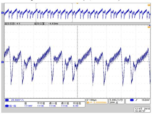
Figure 16. 115-V AC/60-Hz Input, 5-V/5-A Output
