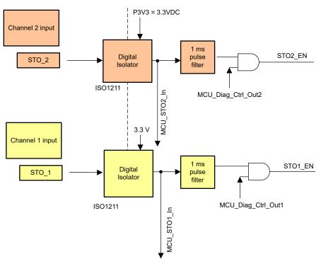
Figure 2-2. Dual-Channel Isolated STO
