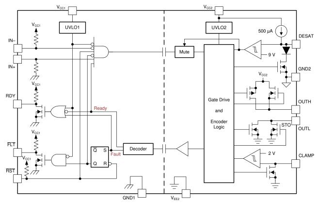
Figure 2-9. ISO5852S, ISO5452 Functional Block Diagram
