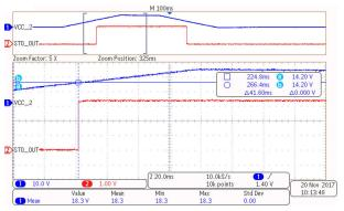
Figure 3-4. Logic Thresholds for Digital Isolator— Rising Edges
