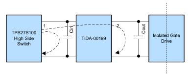
Figure 3-17. Charging of Input and Output Capacitors of TIDA-00199
