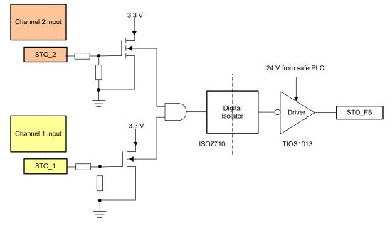
Figure 2-5. STO\_FB Feedback Monitor Subsystem
