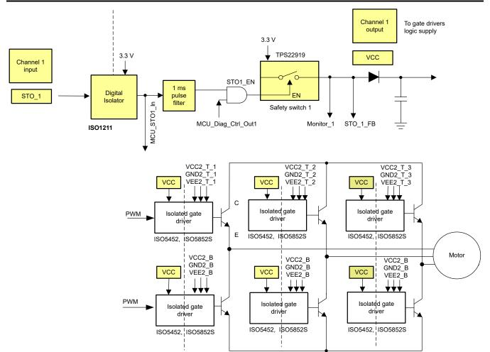
Figure 2-3. STO\_1 Signal Flow Path
