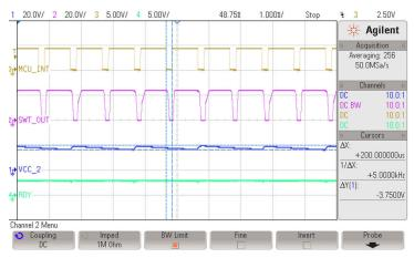
Figure 3-14. Effect of Diagnostic Pulses From MCU Interface on STO2 Signal Path
