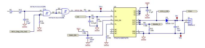
Figure 2-12. TPS27S100 Schematic
