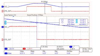
Figure 3-3. Logic Thresholds for Digital Isolator— Falling Edges
