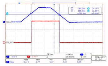
Figure 3-2. Logic Threshold for Digital Isolator
