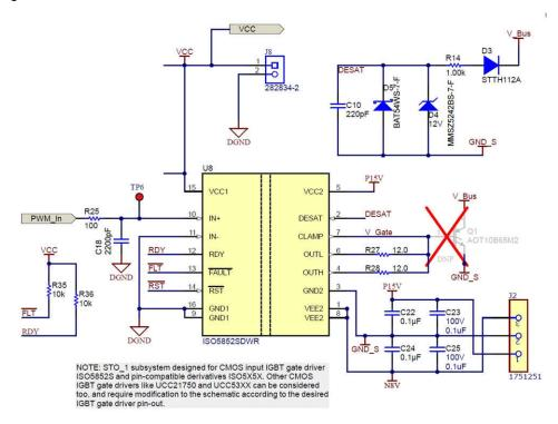
Figure 2-13. ISO5852S Schematic
