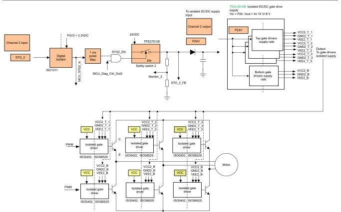
Figure 2-4. STO\_2 Signal Flow Path
