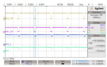
Figure 3-9. Effect of Diagnostic Pulses From MCU Interface on STO1 Signal Path
