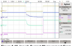
Figure 3-15. Inrush Current Measurement From TPS27S100
