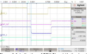
Figure 3-6. Indication of RDY Signal (Active Low) When VCC\_1 Turns OFF
