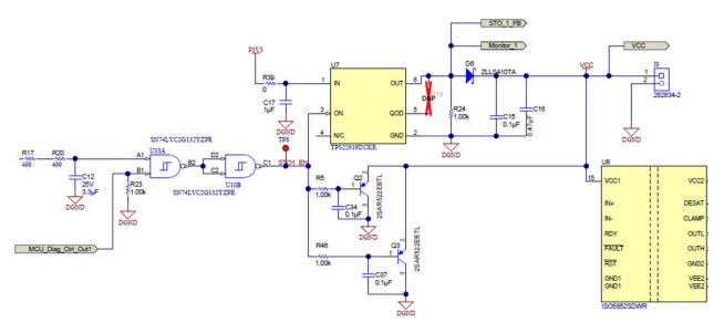
Figure 2-11. TPS22919 Schematic
