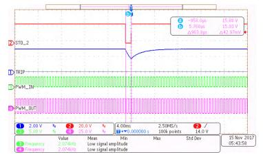
Figure 3-25. Effect of Rejection: 1-ms Pulse on Trip
