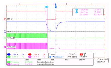
Figure 3-24. Validation of Trip Zone Functionality Through STO2
