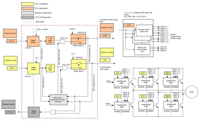
Figure 2-1. System Block Diagram With TIDA-01599
