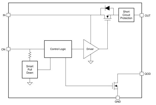
Figure 2-8. TPS22919 Functional Block Diagram
