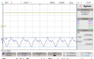
Figure 3-21. Zoomed-in Ripple Voltage at Load Current of 40 mA
