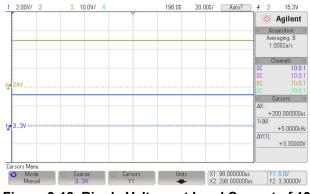
Figure 3-18. Ripple Voltage at Load Current of 13 mA
