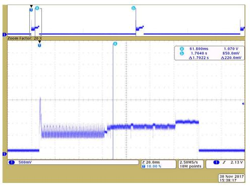
Figure 5. System Current Consumption
