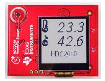
Low-Power, High-Accuracy Temperature and Humidity Meter Reference Design
