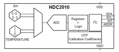
Figure 3. HDC2010 Functional Block Diagram
