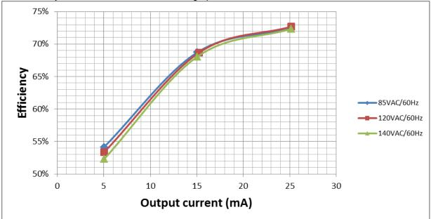
The efficiency data is shown in the tables and graph below. R5=4.7 $\Omega$  in this test.
