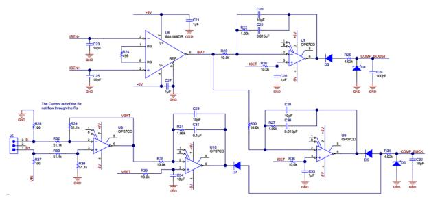
Figure 4: Current and Voltage Control Circuitry
