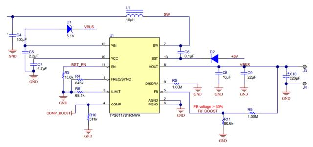
Figure 2: Schematic of TPS61178x
