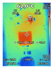
Figure 3: TPS54821 Thermal at 6A operation
