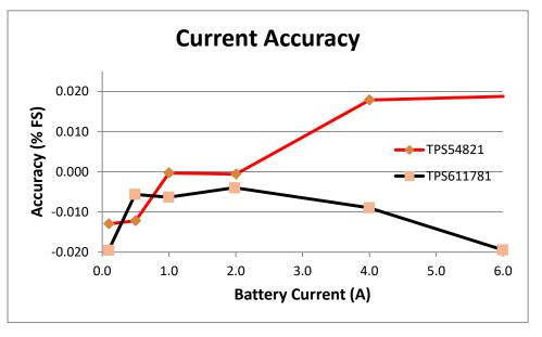
Figure 1: Battery Charge and Discharge Current Accuracy
