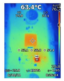
Figure 2: TPS611781 Thermal at 6A operation
