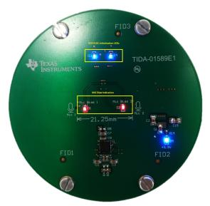
Blue LEDs D3 and D4 on MIC board will illuminate indicating a successful initialization of the TLV320ADC3101 as shown in Figure 33
