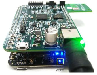
• The Blue power LED on the MIC board indicates the power on the board as Figure 31 shows.
