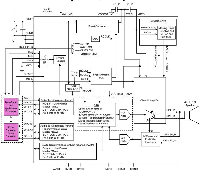
Figure 12. TAS2557 Block Diagram
