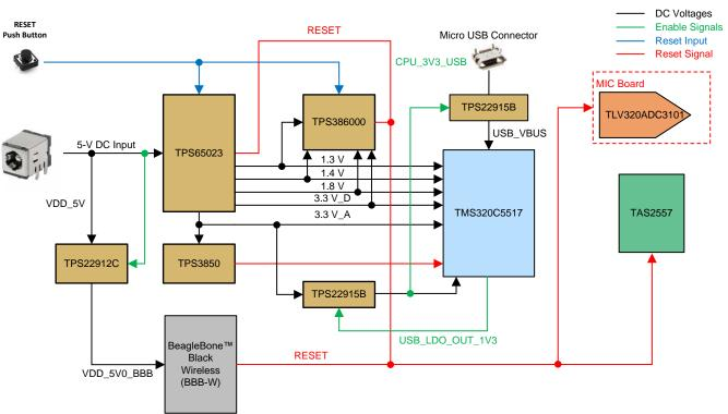
Figure 9. Reset and Power Sequencing
