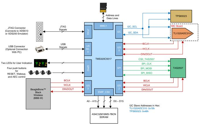
Figure 10. Externals Interfaces With C5517 DSP
