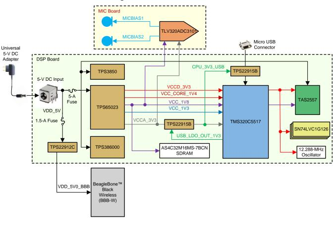
**NOTE:** The BeagleBone Black Wireless (BBB-W) gets power from the TIDA-01589 DSP board so there is no need to connect a DC adapter to BBB-W. The TPS22912C load switch with full time reverse current blocking powers the BBB-W with 5-V DC input from the DSP board.
