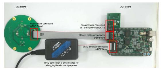
NOTE: The JTAG connection with the DSP board is not required to run the demonstration. It is only required for debugging and development purposes.
