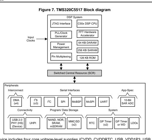
The device includes four core voltage-level supplies (CVDD, CVDDRTC, USB\_VDD1P3, USB\_VDDA1P3), and several I/O supplies including—DVDDIO, DVDDEMIF, DVDDRTC, USB\_VDDOSC, and USB\_VDDA3P3. Figure 8 highlights the set of peripherals available on the C5517 DSP used in this design and their I/O Power supplies:
