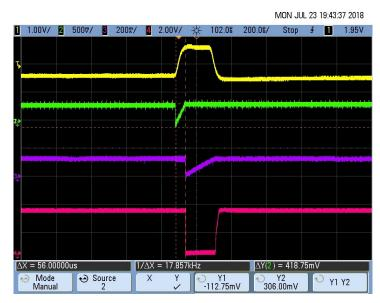
Figure 58. Pacemaker Detection Output (Rise Time T<sub>R</sub>) for 8-mV, 200-µs Pace Pulse
