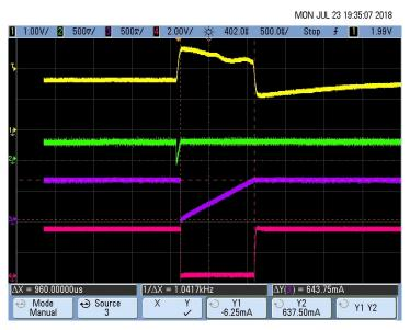
Figure 63. Pacemaker Detection Output (Pulse Duration T<sub>D</sub>) for 8-mV, 1-ms Pace Pulse
