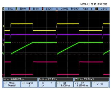
Figure 55. Pacemaker Detection Output for 8-mV, 100-µs Pace Pulse
