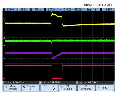
Figure 61. Pacemaker Detection Output (Pulse Duration T<sub>D</sub>) for 8-mV, 500-µs Pace Pulse
