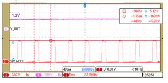
The following figures show the switch node performance of the buck converter, TPS62125, generating 5 V, 8 V, and 10 V for encoder supply.
