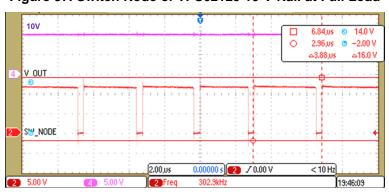
Figure 37. Switch Node of TPS62125 10-V Rail at Full Load
