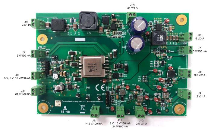
The TIDA-010009 is a compact board with 114-mm x 77.47-mm dimensions. Table 2 provides details on the connectors used in the design.
