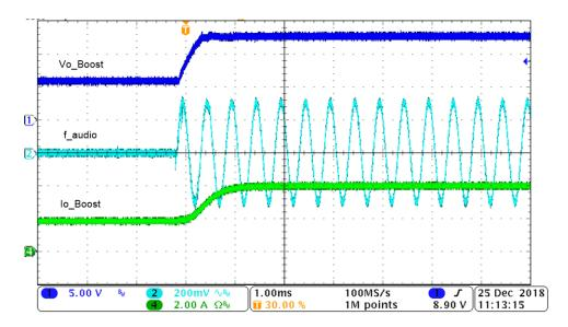
Figure 7. Output Voltage Transition at f\_audio = 2 kHz
