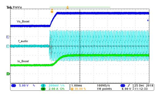
Figure 6. Output Voltage Transition at f\_audio = 20 kHz
