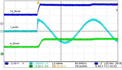
Figure 9. Output Voltage Transition at f\_audio = 100 Hz
