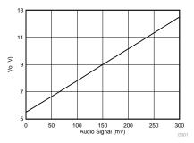
Figure 4. V<sub>out</sub> vs Audio Signal (One-cell)
