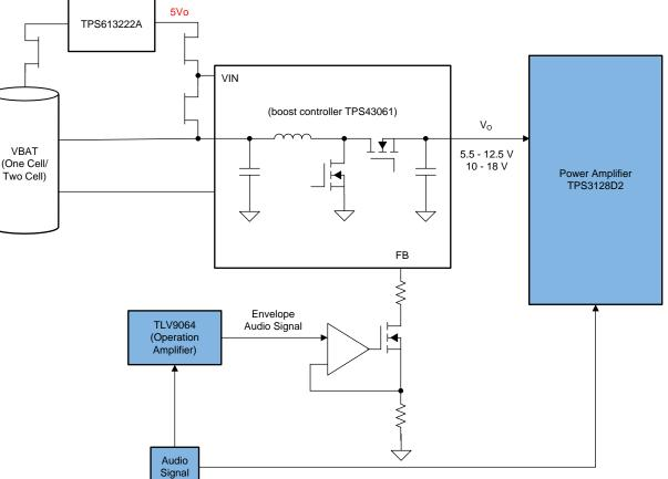
One cell battery: TPS43061's Vin pin connects to the 5V output of TPS613222A; Two cell battery: TPS43061's Vin pin connects to Battery.
