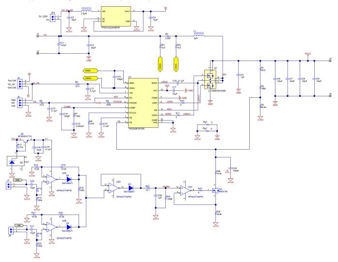
Figure 2. Schematic of TIDA-050024 (Boost Converter)
