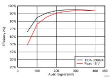
Figure 14. Efficiency Comparison Result with TPA3126D2 (V<sub>IN</sub> = 7.2 V, R<sub>OUT</sub> = 2  $\Omega$ )
