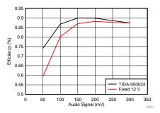
Figure 11. Efficiency Comparison Result With TPA3128D2 (V<sub>IN</sub> = 3.75 V, R<sub>out</sub> = 2  $\Omega$ )
