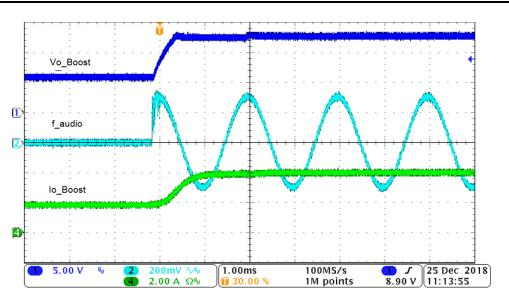
Figure 8. Output Voltage Transition at f\_audio = 500 Hz
