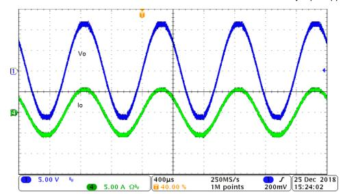
Figure 15 shows the waveforms across a 2- $\Omega$  load at the one-cell Lithium battery-input application.
