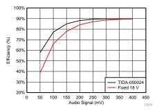
Figure 12. Efficiency Comparison Result With TPA3128D2 (V<sub>IN</sub> = 7.2 V, R<sub>OUT</sub> = 3  $\Omega$ )
