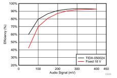
Figure 13. Efficiency Comparison Result With TPA3126D2 ( $V_{IN}$  = 7.2 V,  $R_{OUT}$  = 3  $\Omega$ )
