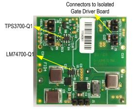
Figure 13 shows the LM5180-Q1 based flyback PCB board implemented on top of the isolated gate driver board and the IGBT module.
