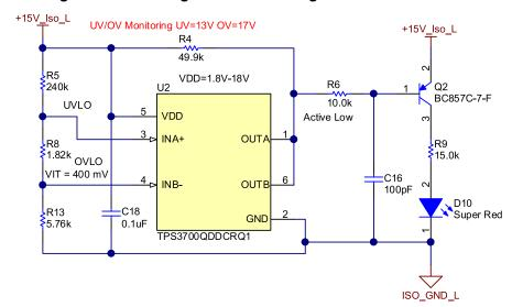
Figure 9. Overvoltage and Undervoltage Detection Schematic
