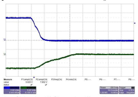
Figure 21. Power Down Waveform of the -9-V Rail With  $V_{IN} = 5$  V and no Load
