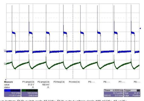
Figure 29. Switch Node and Output Ripple of the -9-V Rail with  $V_{\rm IN}=5$  V and 85-mA Load
