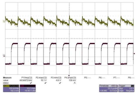
Figure 49. Voltage Ripple of the -9-V Rail While Switching the IGBT Module at 50 kHz
