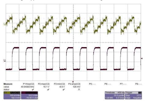
Figure 48. Voltage Ripple of the 15-V Rail While Switching the IGBT Module at 50 kHz
