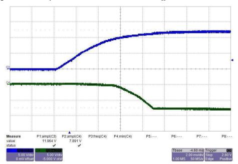
Figure 19. Start-up Waveform of the -9-V Rail With  $V_{IN} = 12 V$  and 180-mA Load
