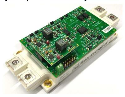
Figure 13. Implementation With Power Stage and IGBT Module
