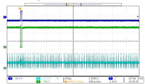
Figure 53. CMTI Test With Double Pulses
