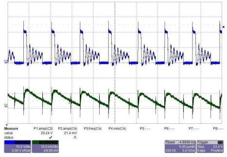
From top to bottom: CH3: switch node 10 V/div, CH4: output voltage ripple 10 mV/div, 5 µs/div
