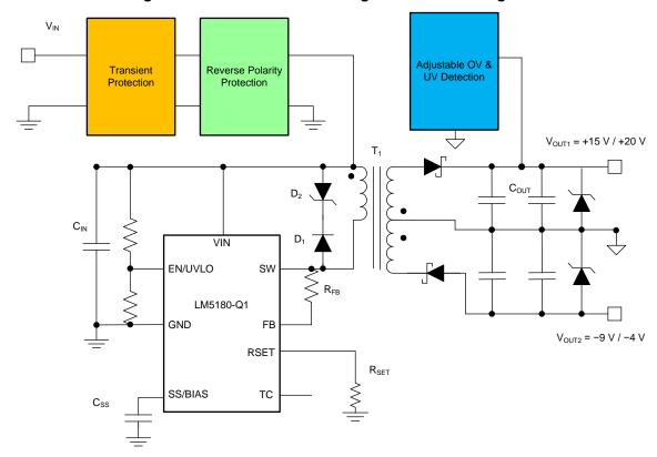
Figure 2. TIDA-020015 Low-Voltage Board Block Diagram
