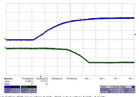
Figure 17. Start-up Waveform of the –9-V Rail With  $V_{\rm IN}$  = 12 V and no Load
