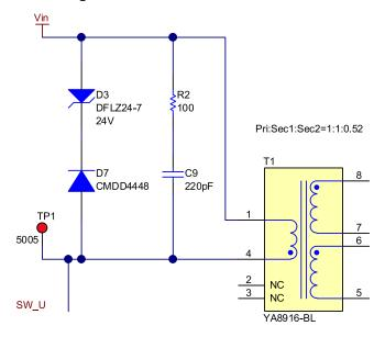
Figure 7. Snubber Circuit Schematic
