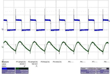
From top to bottom: CH3: switch node 20 V/div, CH4: output voltage ripple 100 mV/div, 5 µs/div
