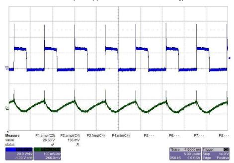
Figure 33. Switch Node and Output Ripple of the -9-V Rail With  $V_{\rm IN}=12~V$  and  $180-{\rm mA}$  Load
