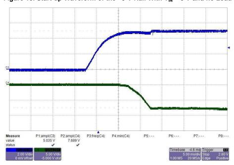
Figure 15. Start-up Waveform of the -9-V Rail With  $V_{IN} = 5$  V and no Load
