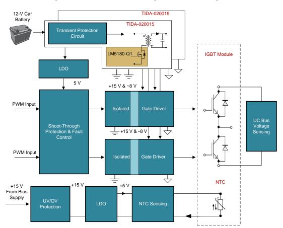
Figure 3. TIDA-020015 Power Stage Board Block Diagram
