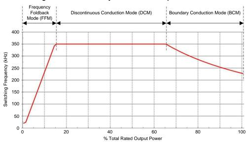
Figure 6. LM5180-Q1 Flyback Converter Operation Mode
