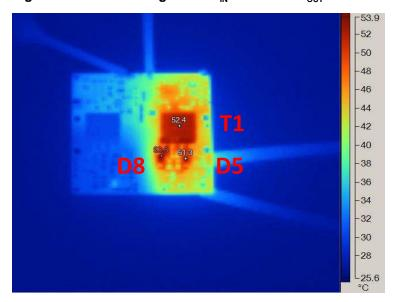
Figure 50. Thermal Image With  $V_{\rm IN}$  = 12 V and  $I_{\rm OUT}$  = 180 mA
