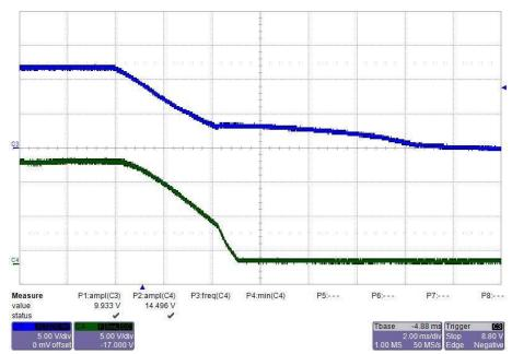
Figure 25. Power Down Waveform of the +15-V Rail With  $V_{IN}$  = 12 V and 180-mA Load
