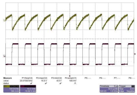
From top to bottom: CH1: output voltage 100 mV/div, CH2: gate PWM signal 10 V/div, 50 µs/div
