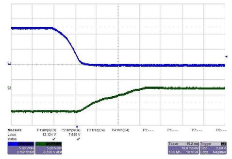
From top to bottom: CH3: input voltage 5 V/div, CH4: output voltage 5 V/div, 10 ms/div
