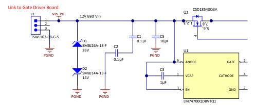
Figure 4. Reverse Polarity Protection Circuit Schematic
