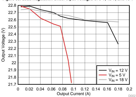
Figure 39. Load Regulation Under Input Voltages of 5 V, 12 V, and 18 V
