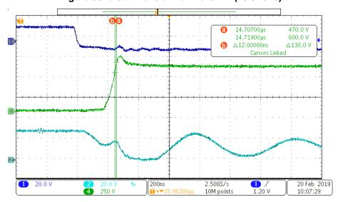
Figure 55. dv/dt Transient of the CMTI (10.8 V/ns)
