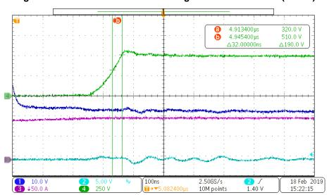
Figure 52. dv/dt at the IGBT Vds Voltage Turn-off Transient (6 V/ns)
