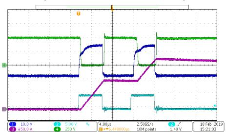
Figure 51. Double Pulse Test on the Power Stage
