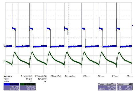
From top to bottom: CH3: switch node 10 V/div, CH4: output voltage ripple 100 mV/div, 10  $\mu$ s/div
