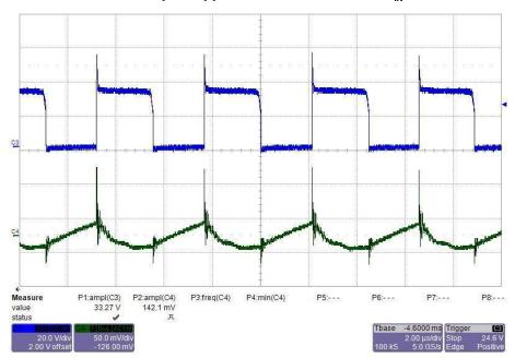
Figure 37. Switch Node and Output Ripple of the -9-V Rail With  $V_{\rm IN}=18~V$  and  $180-{\rm mA}$  Load
