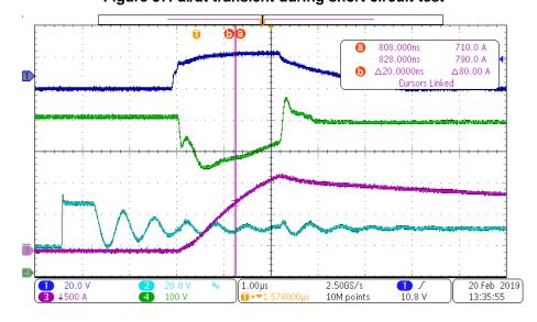
Figure 57. di/dt transient during short circuit test
