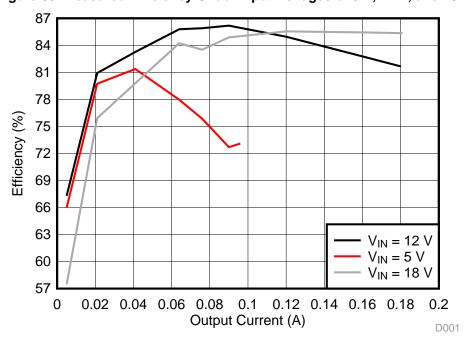
Figure 38. Measured Efficiency Under Input Voltages of 5 V, 12 V, and 18 V
