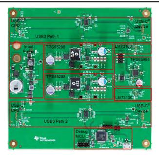
Figure 2-2. PCB Subsection Overview
