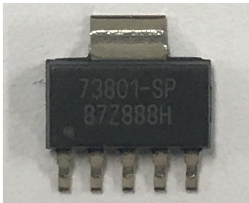
Figure 1. TPS73801-SEP Device Photo
