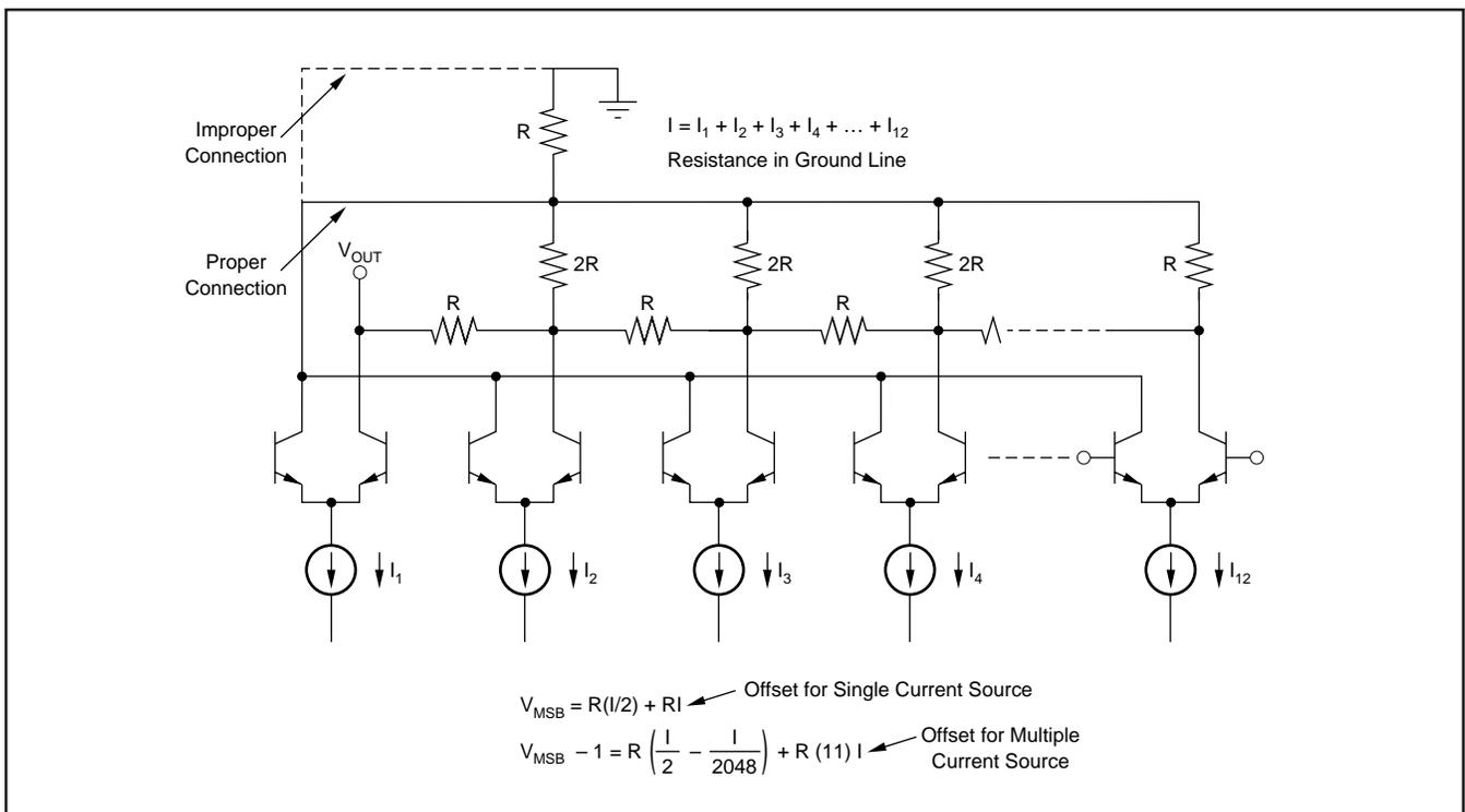
FIGURE 64. Superposition Error.
