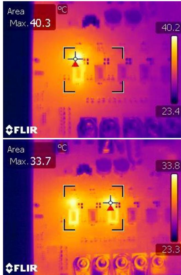
The single phase solution is running almost 7°C hotter than the dual phase configuration for the same conditions! Multiphase thermal performance will only improve as the load current increases to 30A and beyond. Sticking with single phase for such high currents quickly leads to a complicated thermal design as heftier heatsinks and more airflow is required to keep the FETs at a safe operating temperature.
