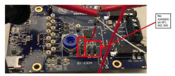
Figure 5. EVM Board With No Jumpers
