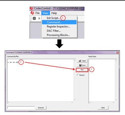
Figure 7. Enabling Headset Detection Using Command
