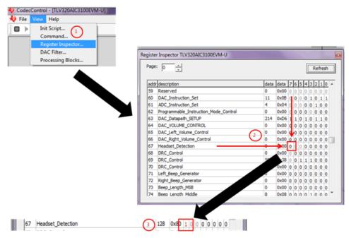
Figure 6. Enabling Headset Detection Using Register Inspector
