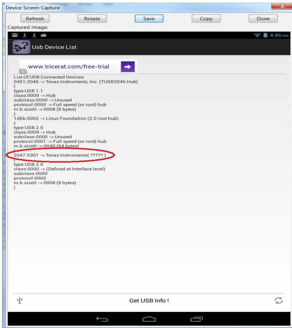
Figure 3. Enumerated HID Device With VID/PID (2047/301)
