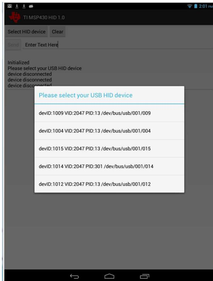
**Figure 5. List of VID/PID of Connected USB Devices**
