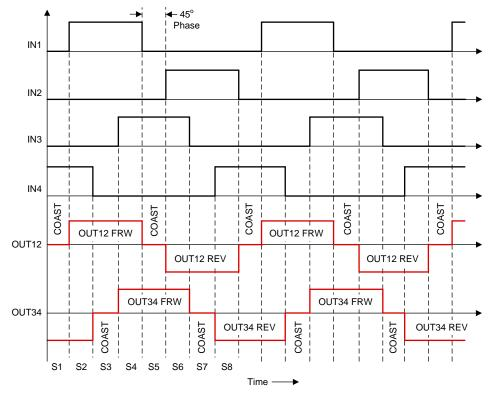
Figure 15. Waveforms for Stepper Motor Operation in Half Step Mode (with Hi-Z Off State)
