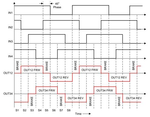
Figure 25. Waveforms for Stepper Motor Operation in Half Step Mode (with Brake Off State)
