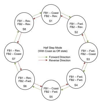
Figure 16. Sequence Chart for Stepper Motor Operation in Half Step Mode (with Hi-Z Off State)
