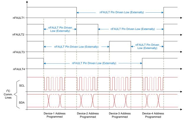
Figure 29. Multi-Slave Operation Waveforms
