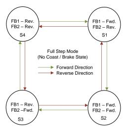
Figure 6. Sequence Chart for Stepper Motor Operation in Full Step Mode
