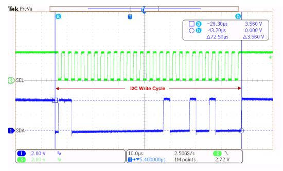
Figure 31. DRV8847S Single Register I<sup>2</sup>C Write Latency
