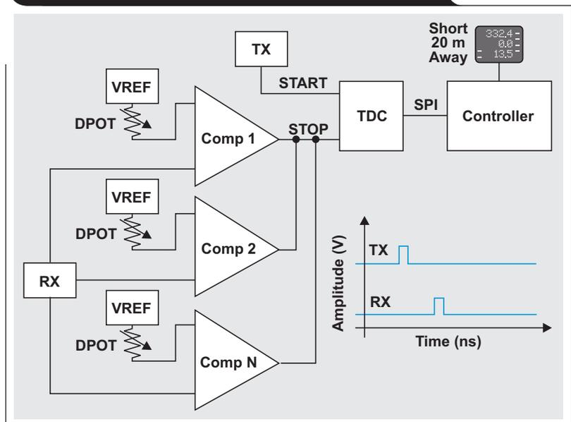
Figure 3. Cable diagnostics block as part of a MDI layer
