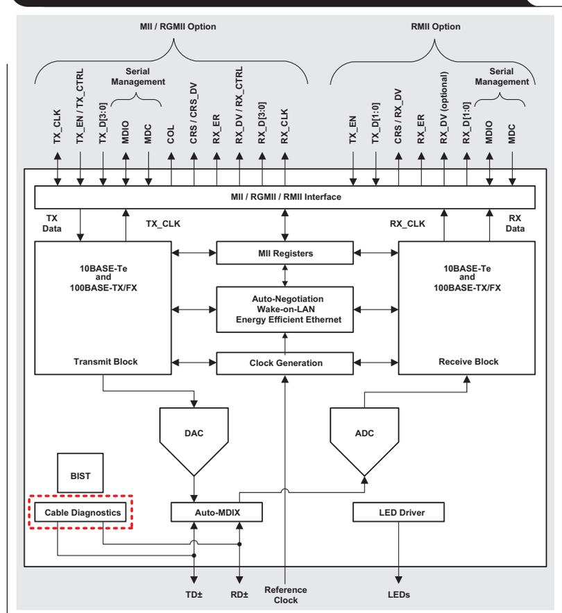
The microcontroller (MCU) host configures, starts, and reads out results through the management-data input/output (MDIO) and management-data clock (MDC) interface between the MCU and Ethernet PHY. The cable-diagnostic function is part of the extended register space within the PHY and is accessed over the MDIO function block inside the MCU host. This is shown in Figure 4.
