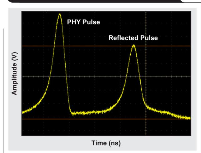
**Figure 6. Example of a TDR pulse measuring a shorted-cable fault**
