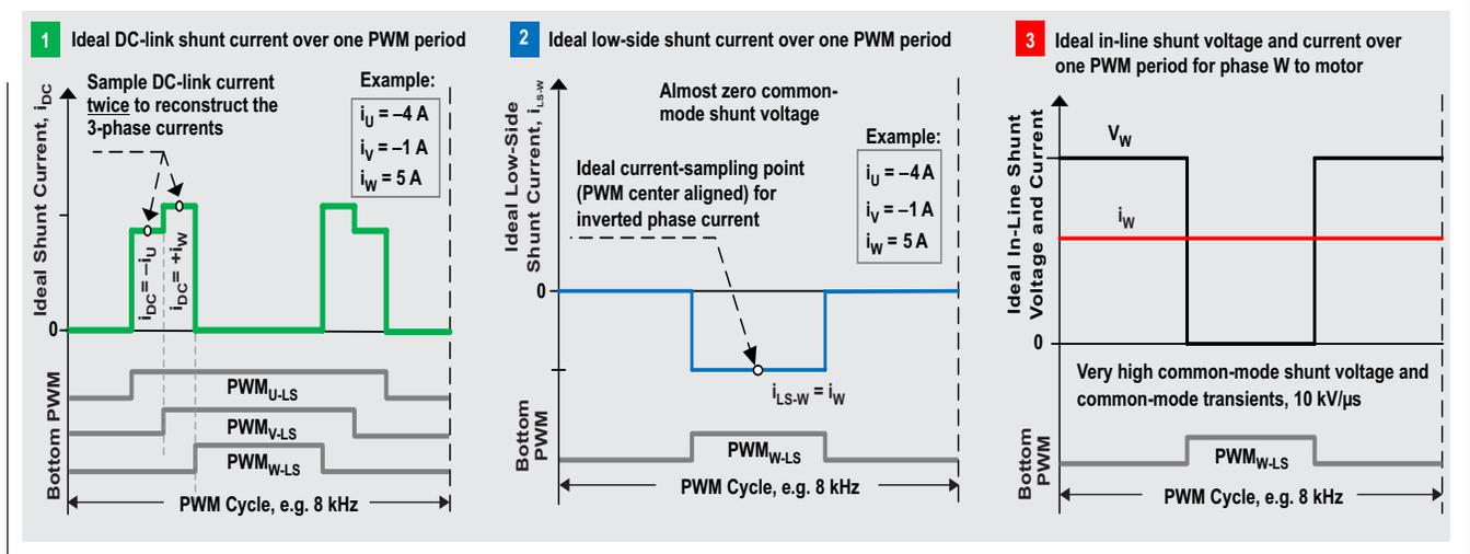
**Table 1. Comparison of shunt placement for motor phase-current measurement**
