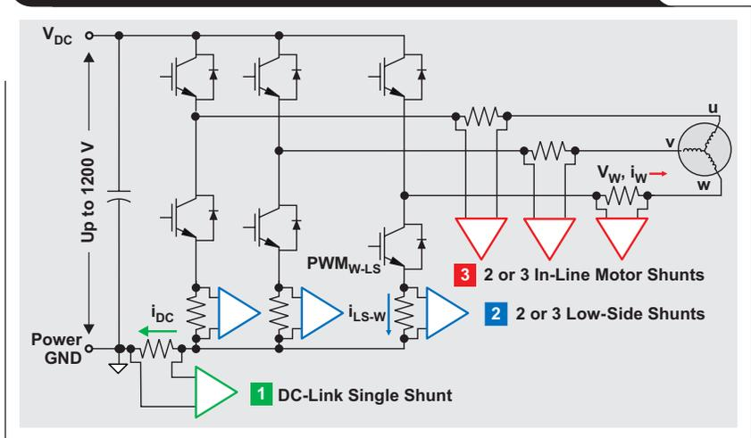
Figure 2. Shunt current vs. phase current and common mode depending on shunt placement
