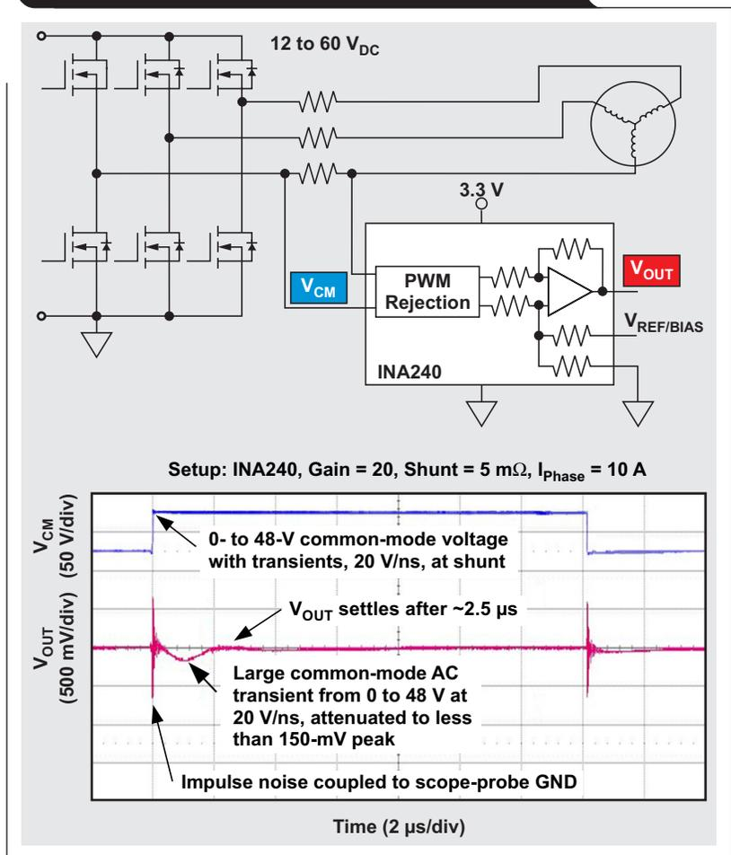
**Isolated in-line phase-current sensing**
