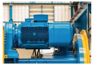
*Figure 1.* Induction motor with an AC motor drive in a factory. An AC motor drive takes an AC energy source, rectifies it to a DC bus voltage and, implementing complex control algorithms, inverts the DC back to AC into the motor via complex control algorithms based on load demand.
