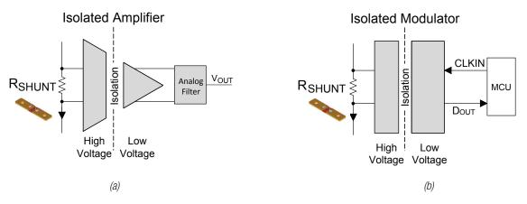
Figure 4. Examples of an isolated amplifier (a); and isolated modulator (b).
