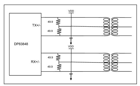
Figure 2. DP83848C/I/YB PMD Connections (Termination)
