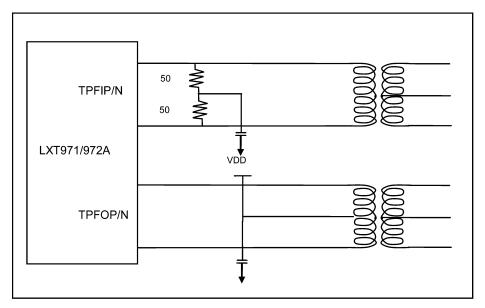
Figure 3. LXT971 and LXT972A PMD Connections (Termination)
