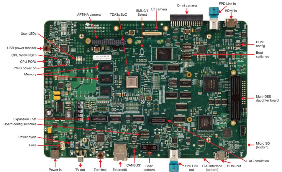
▲ Figure 3. TDA3x Evaluation Module with imager interfaces
