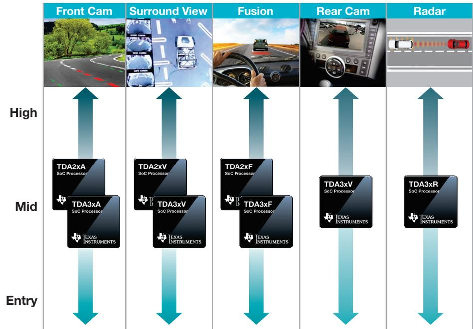
▲ Figure 1: Scalability between TDA2 and TDA3x SoCs for various ADAS applications
