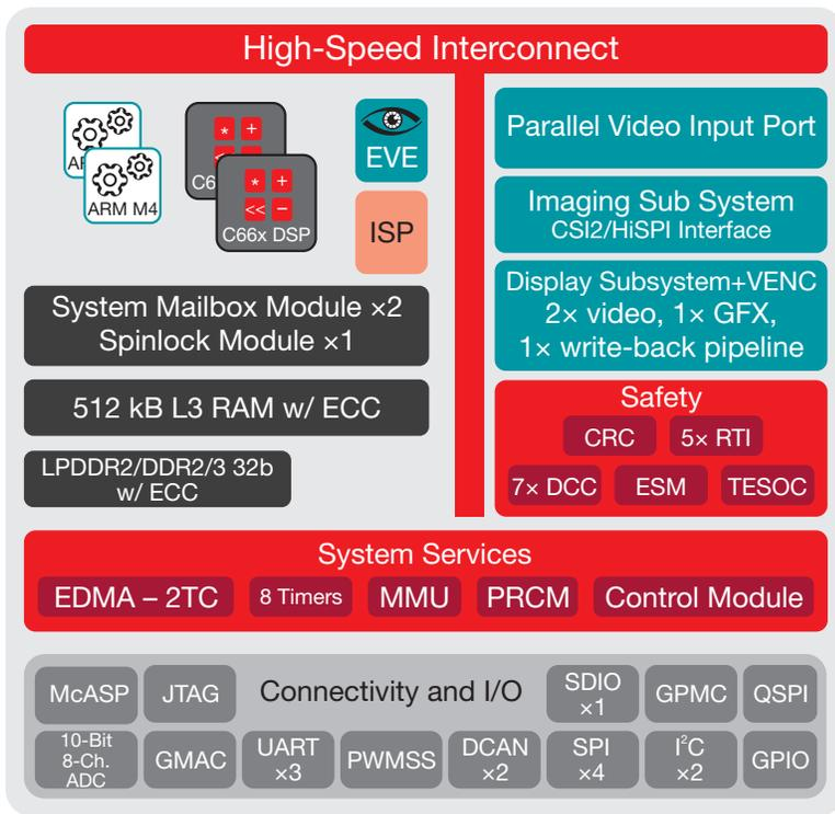
▲ Figure 2: TDA3x SoC block diagram
