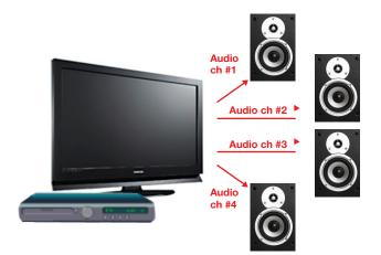
Up to four devices streaming one out of four audio channels. Example: Multi-room system where two speaker sets play different stereo audio streams.
