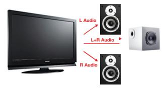
Each device can selectively receive one or two of the transmitted audio streams. Example: 2.1 speaker system
