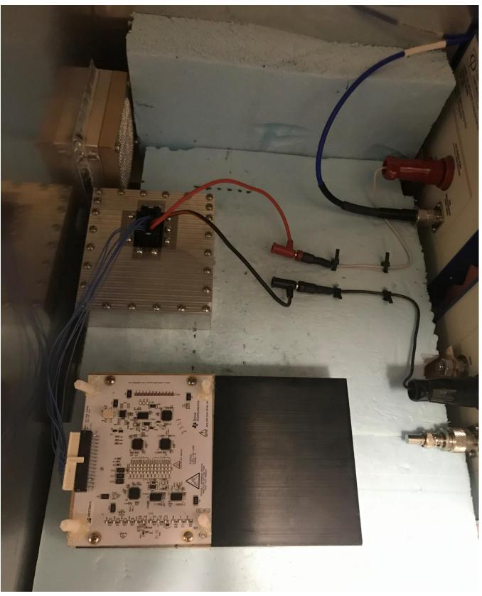
Figure 32. CISPR 25 Conducted Emissions Connections
