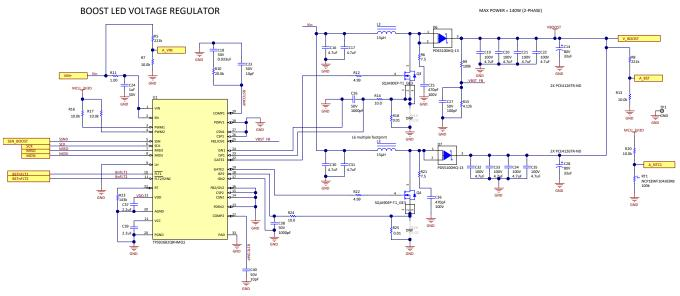
Figure 9. Schematic of TPS92682-Q1 Boost Controller
