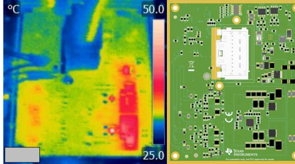
Figure 23 shows temperatures at various sample points (Sp). Figure A shows that most of the power dissipation is contained within the boost converter section of the design. Sp1 is the case temperature of the TPS92682-Q1. Sp2 and Sp3 are temperatures at the current sense resistors (R25 and R18). Sp5 is the temperature for the current sense resistor of for VBUCK1 (R42). Sp4 and Sp6 are the temperatures next to Q3, D6, Q4, and D7.
