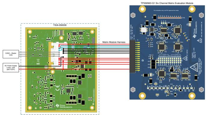
Figure 27 shows the connection points for the TIDA-050030 connector to the TPS92663-Q1 six channel matrix evaluation module.
