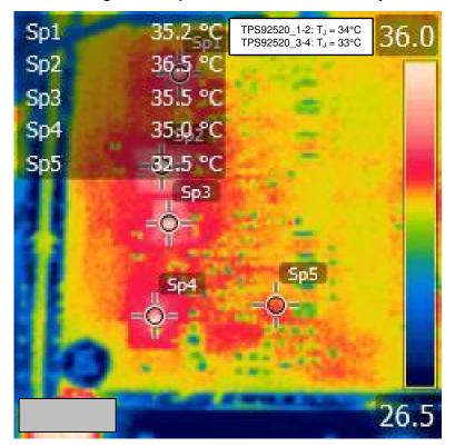
Figure 25. Thermal Image: Closeup of Buck Converter Circuitry at ≈ 120 W Output
