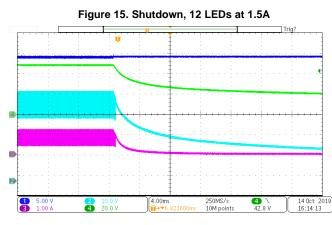
CH1: VIN, CH2: VOUT LED driver, CH3: LED current, CH4: VBOOST
