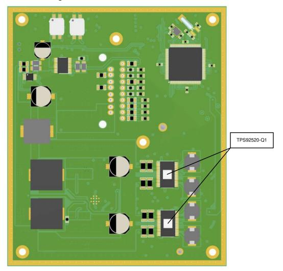
Figure 7. 3D Render of TIDA-050030 PCB-Bottom Side
