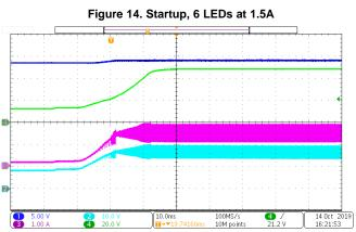
CH1: VIN, CH2: VOUT LED driver, CH3: LED current, CH4: VBOOST
