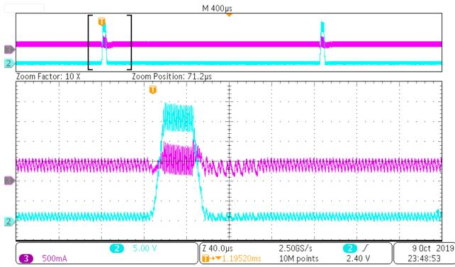
Figure 29. Waveforms of 0 Phase Shift, 1000/1024 Pulse Width, SLEWRATE=01, at 350mA Using Lighting Matrix Module EVM
