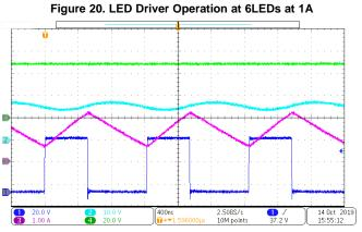
CH1: SW LED driver, CH2: VOUT LED driver, CH3: IL LED, CH4: VBOOST
