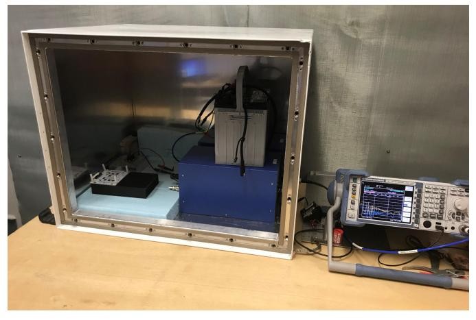
Figure 31. CISPR 25 Conducted Emissions Setup
