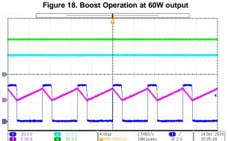
CH1: SW boost, CH2: VIN, CH3: IL boost, CH4: VBOOST (NOTE: only one of two phases)
