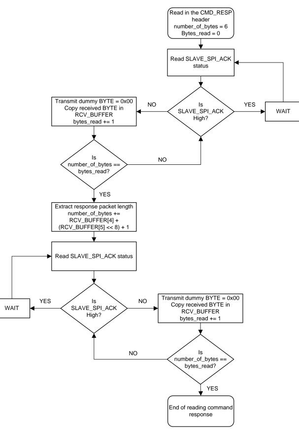
Figure 3. Read Command Response Flowchart
