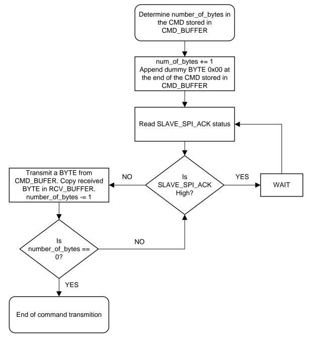
Figure 2. Write Command Transmit Flowchart
