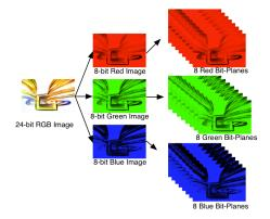
Figure 2-5. Bit-Planes of a 24-Bit RGB Image
