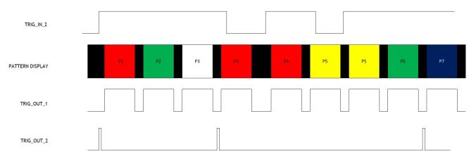
Figure 2-10. Trigger Mode 1 Timing Diagram Example
