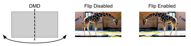
Figure 2-1. Image Long-Axis Flip Example
