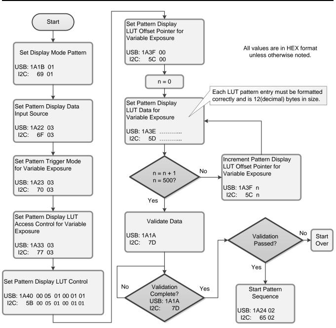
Figure 2-12. Flowchart Example for Programming 1280 Variable Exposures
