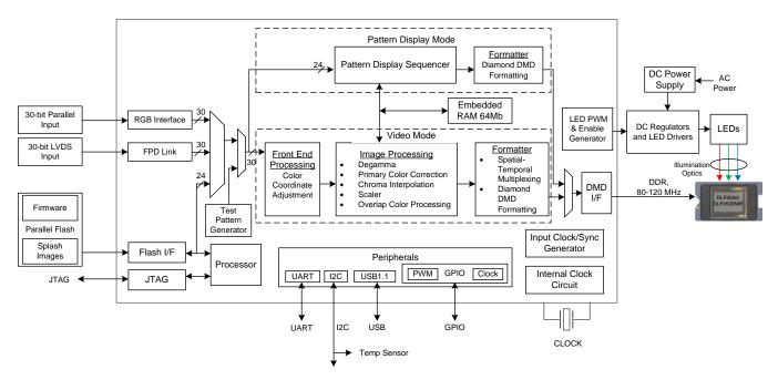
Figure 2-4. DLPC350 Functional Block Diagram
