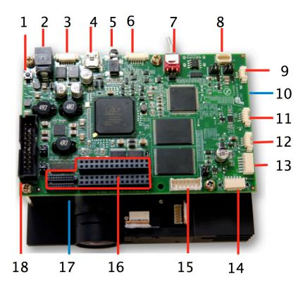
Figure 1-7. DLP LightCrafter 4500 Connectors (Top View)
