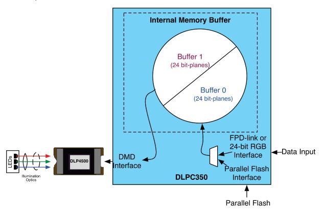
Figure 4-3. DLPC350 Internal Memory Buffer
