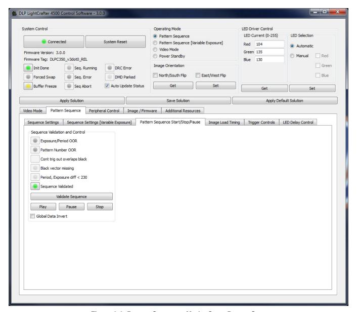
Figure 3-6. Pattern Sequence Mode: Start, Pause, Stop
