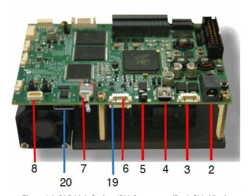
Figure 1-8. DLP LightCrafter 4500 Connectors (Back-Side View)
