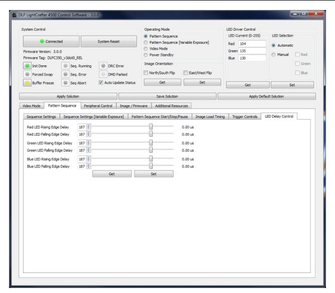
Figure 3-12. LED Delay Control Subtab
