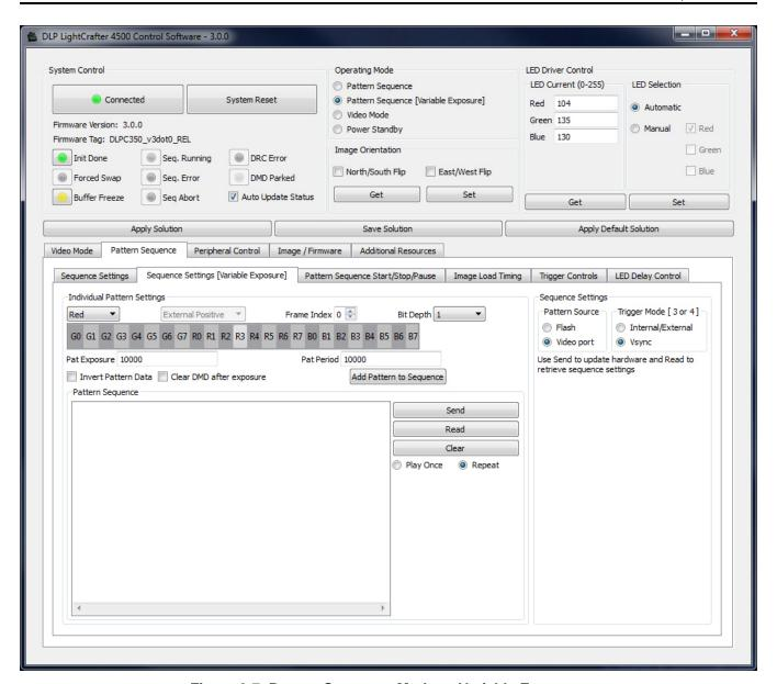
Figure 3-7. Pattern Sequence Mode — Variable Exposure
