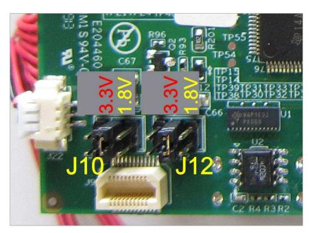
Figure 1-10. DLP LightCrafter 4500 J10 and J12 Voltage Jumpers
