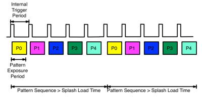
Figure 4-5. Image Load Time and Pattern Sequence Timing
