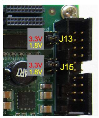
Figure 1-11. DLP LightCrafter 4500 J13 and J15 Voltage Jumpers
