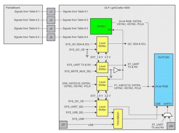
Figure 6-2. Block Diagram of the PandaBoard Interface
