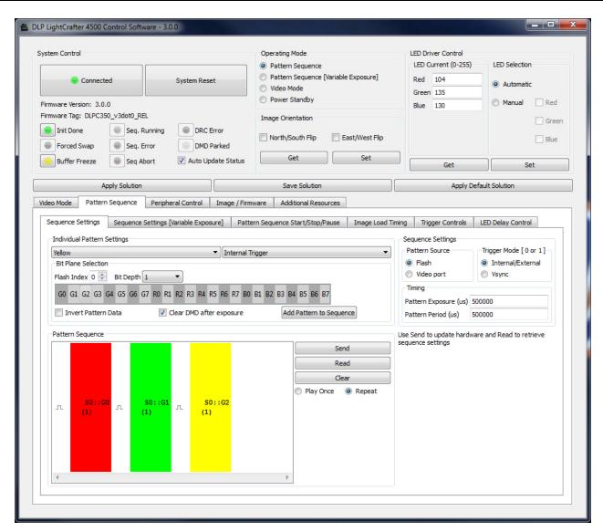
Figure 3-5. DLP LightCrafter 4500 GUI - Pattern Sequence Mode
