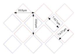
Figure 1-3. 0.45-Inch DMD Diamond Pixel Geometry
