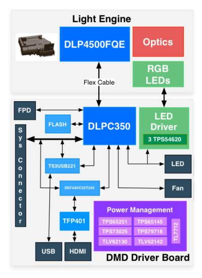
Figure 1-1. DLP LightCrafter 4500 Block Diagram
