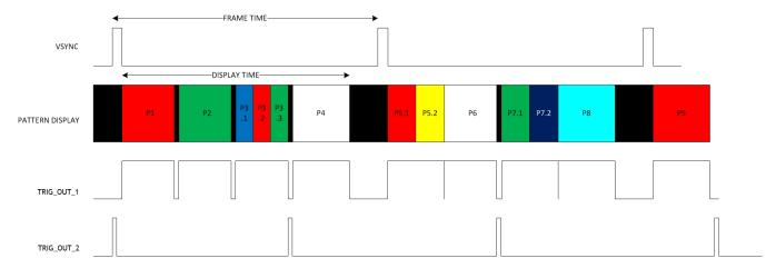
Figure 3-10. VSYNC Pattern Trigger Mode
