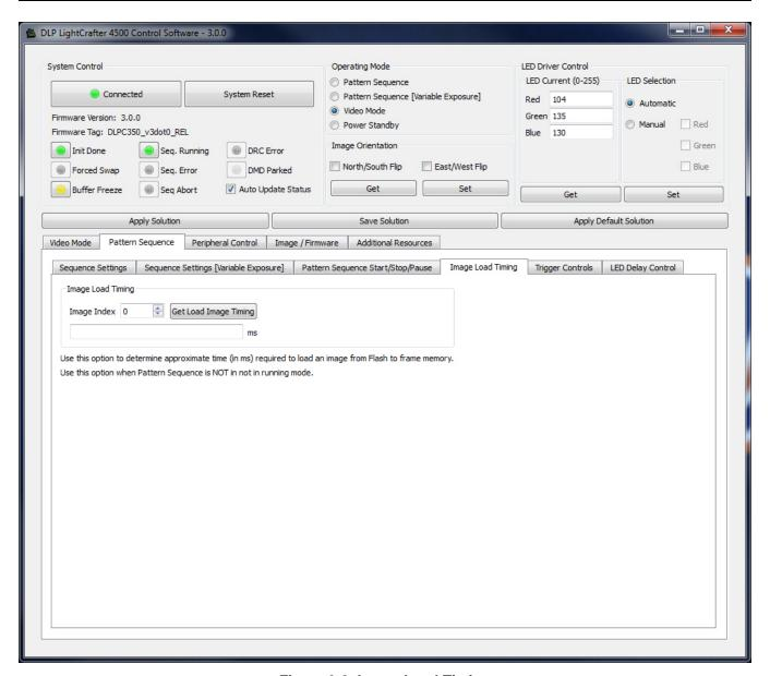
Figure 3-8. Image Load Timing
