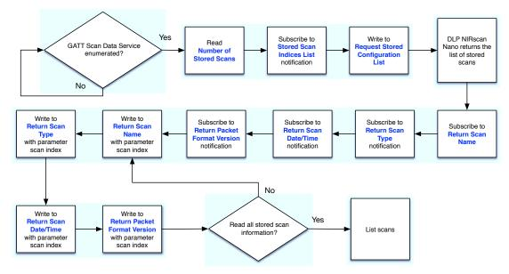
Figure 5-12. GATT Scan Data Service Workflow
