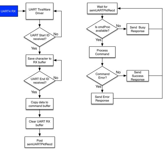
Figure 5-8. UART Command Processing Workflow
