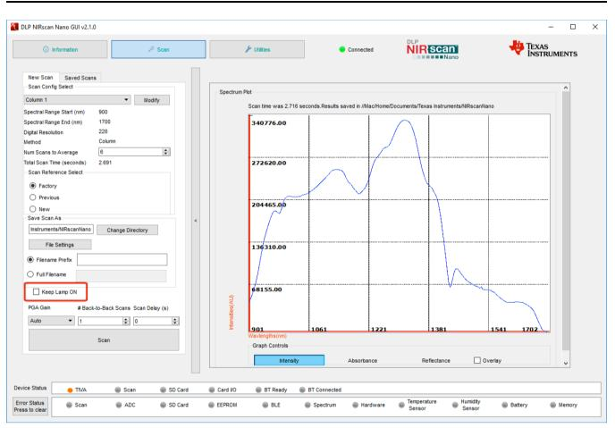
Figure 3-6. DLP NIRscan Nano Keep Lamp On Checkbox
