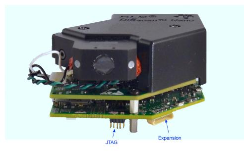
Figure 1-7. DLP NIRscan Nano Connectors (Front View)
