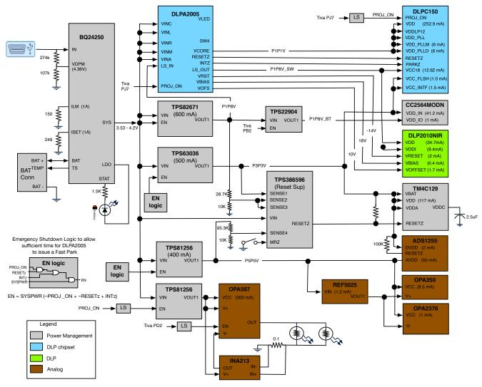
Figure 4-1. DLP NIRscan Nano Power Block Diagram
