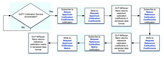
Figure 5-10. GATT Calibration Service Workflow
