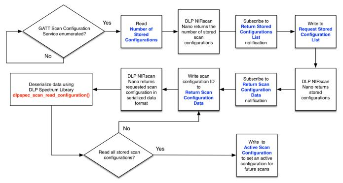
Figure 5-11. GATT Scan Configuration Service Workflow
