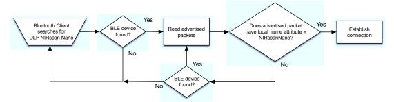
Figure 5-9. Bluetooth Low Energy Connection Workflow
