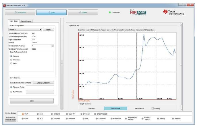
Figure 3-2. DLP NIRscanNano GUI Scan Screen
