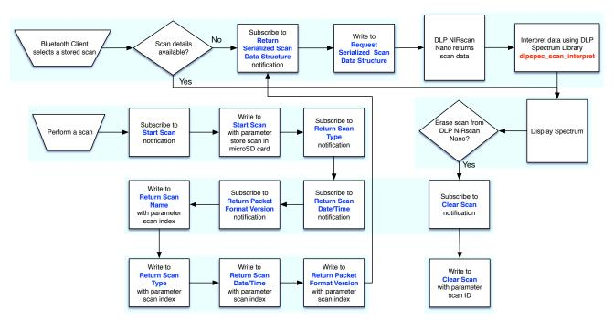
Figure 5-13. GATT Scan Data Service Workflow to Display an Existing Scan or Performing a New Scan
