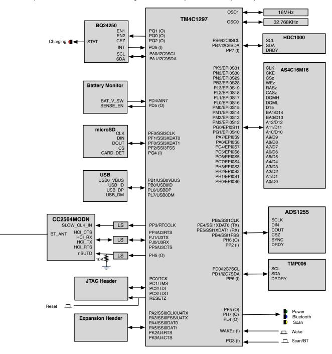
Figure 4-2. DLP NIRscan Nano Tiva Connections
