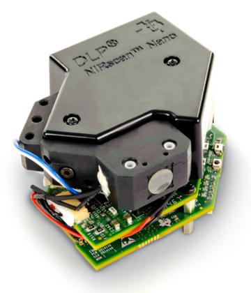
Figure 1. DLP NIRscan Nano Evaluation Module
