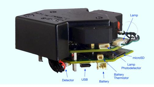
Figure 1-6. DLP NIRscan Nano Connectors (Rear View)
