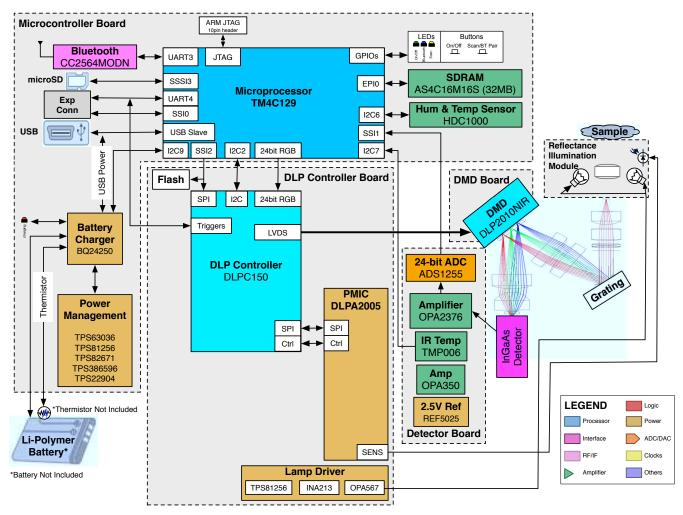
Figure 1-2. DLP NIRscan Nano Block Diagram
