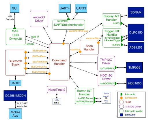
Figure 5-7. DLP NIRscan Nano Software Block Diagram
