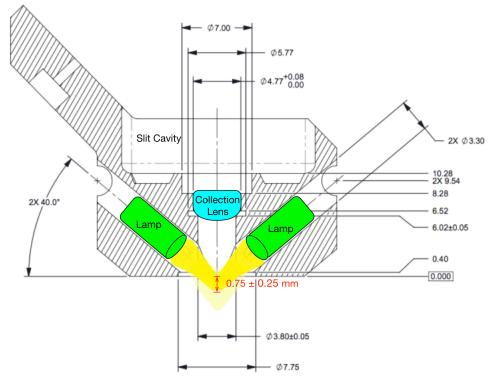
Figure 1-4. Top View for Illumination Module
