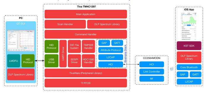
Figure 5-1. DLP NIRscan Nano Software Architecture
