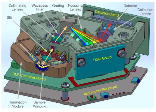
Figure 1-3. DLP NIRscan Nano Optical Engine
