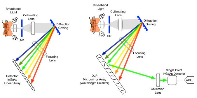
Figure 1-1. Traditional Versus DLP-based Spectrometer
