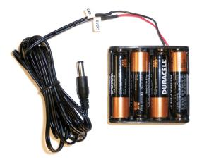
Figure 49. Recommended Power Supply for ADS1x98ECG-FE
