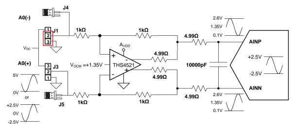
Figure 3. Single-Ended Signal Example
