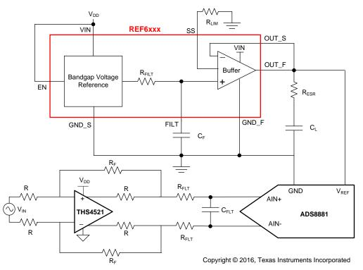
Figure 1. REF6025EVM Schematic Block Diagram
