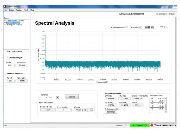
Figure 11. Spectral Analysis Tool
