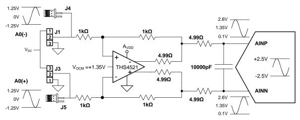
Figure 2. Differential Input Example
