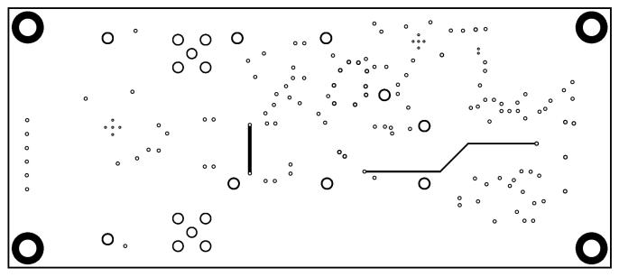
Figure 16. REF6025EVM PCB Layer 4: Bottom Layer
