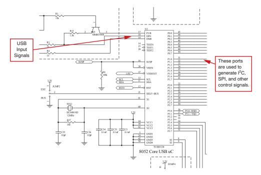
Figure 4. Digital I/O Area—Microcontroller
