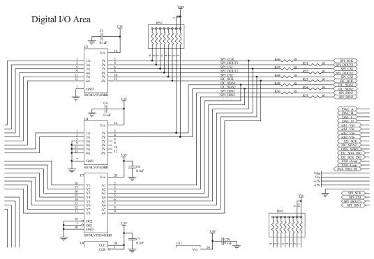
Figure 5. Digital I/O Area—I<sup>2</sup>C and SPI
