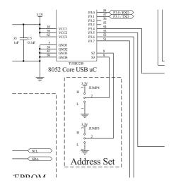
Figure 8. Digital I/O Area—Address Select
