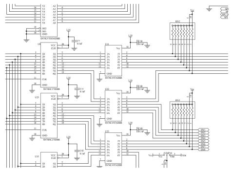
Figure 6. Digital I/O Area—Internal Control Signals
