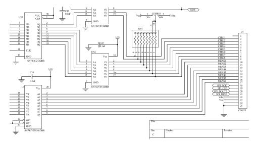
Figure 7. Digital I/O Area—CTRL and MEAS
