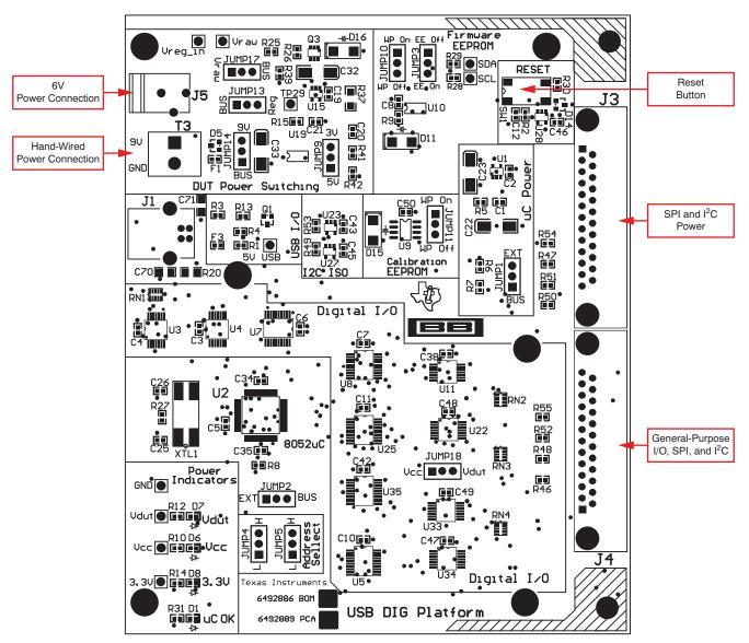
Figure 19. Connector Definition
