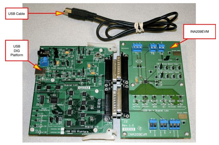
Figure 1 illustrates the typical hardware included the USB DIG Platform.
