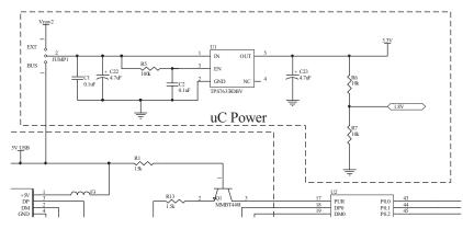
Figure 9. Microcontroller Power
