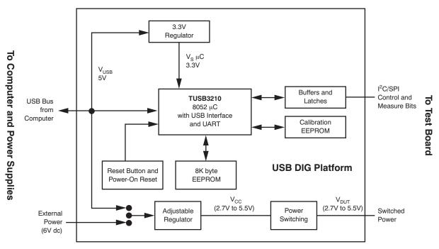
Figure 3. USB DIG Platform Block Diagram
