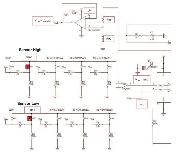
Figure 7. SensorEmulator Section (PGA308 Input)
