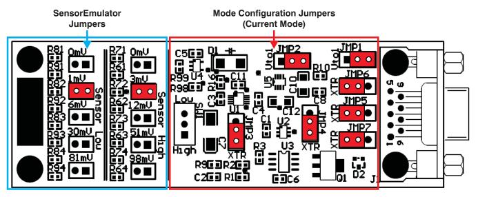
Figure 2. Jumper Settings for Current Output Mode
