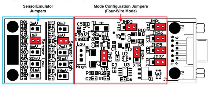
Figure 3. Jumper Setting for Voltage Output Four-Wire Mode
