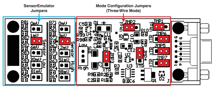
Figure 4. Jumper Setting for Voltage Output Three-Wire Mode
