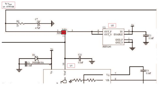
Figure 6. Reference Circuit (Configured for Current Mode)
