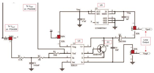
Figure 5. Current Mode Circuit (Configured for Current Mode)
