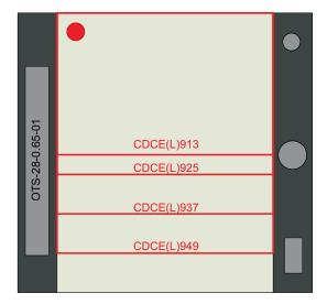
Figure 5. CDCE(L)9xx Device Location in Socket
