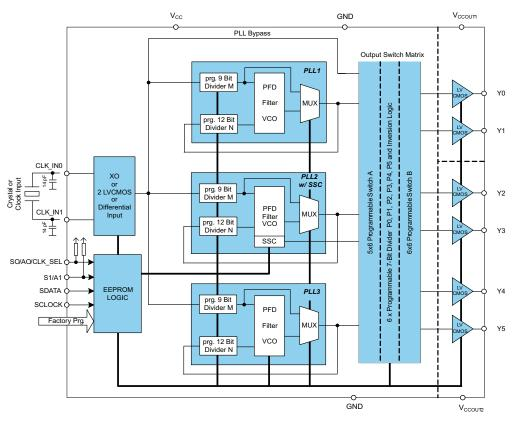
Figure 3. Functional Block Diagram of CDCEx06
