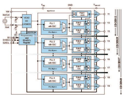
Figure 2. Functional Block Diagram of CDCE(L)9xx
