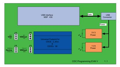
Figure 4. CDCE(L)9xx and CDCEx06 Programming EVM Block Diagram
