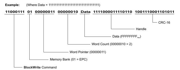
Figure 2-25. BlockWrite Command
