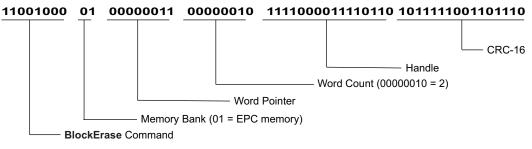
Figure 2-27. BlockErase Command
