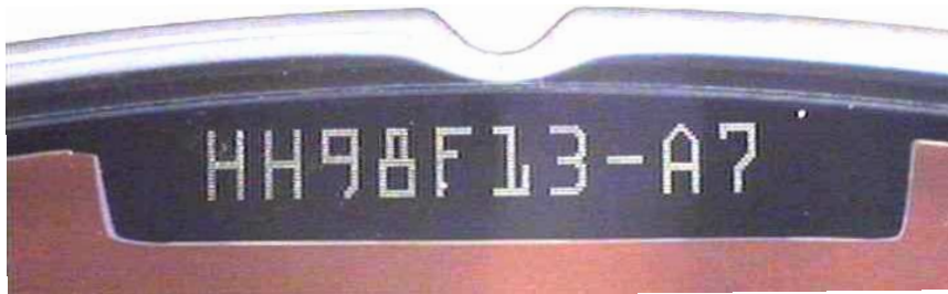
Figure 3-3. Wafer Identification Code 2
