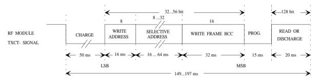
The data format of the Lock Page function is checked by the transponder using the hardware CRC Generator. Lock Page function is executed by the transponder if:
