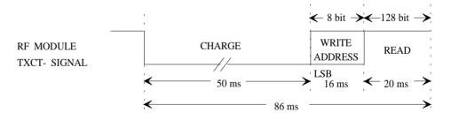
Because the Write Address is not protected by Protection Data, the Sequence Control must check during the Read phase that the correct Page is returned and the Status of the Read Address is valid. The Status of the Read Address must be: Read unlocked Page, or Read locked Page.
