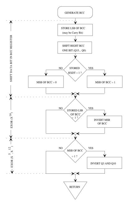
Figure 13: Subroutine 'Generate Block Check Character'
