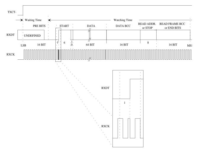
Figure 6: Data Format at the Receiver Outputs
