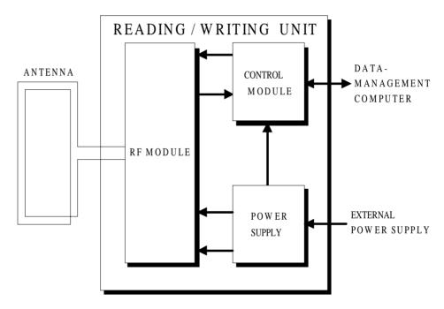
The RF module contains the basic functions to allow data to be read from and written to the transponder. Inductive coupling principle is used for data transmission between the Reading/Writing Unit and the transponder.
