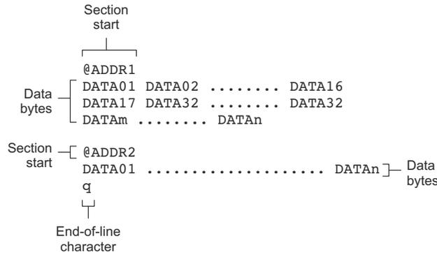
**Figure 12-11. TI-TXT Object Format**
