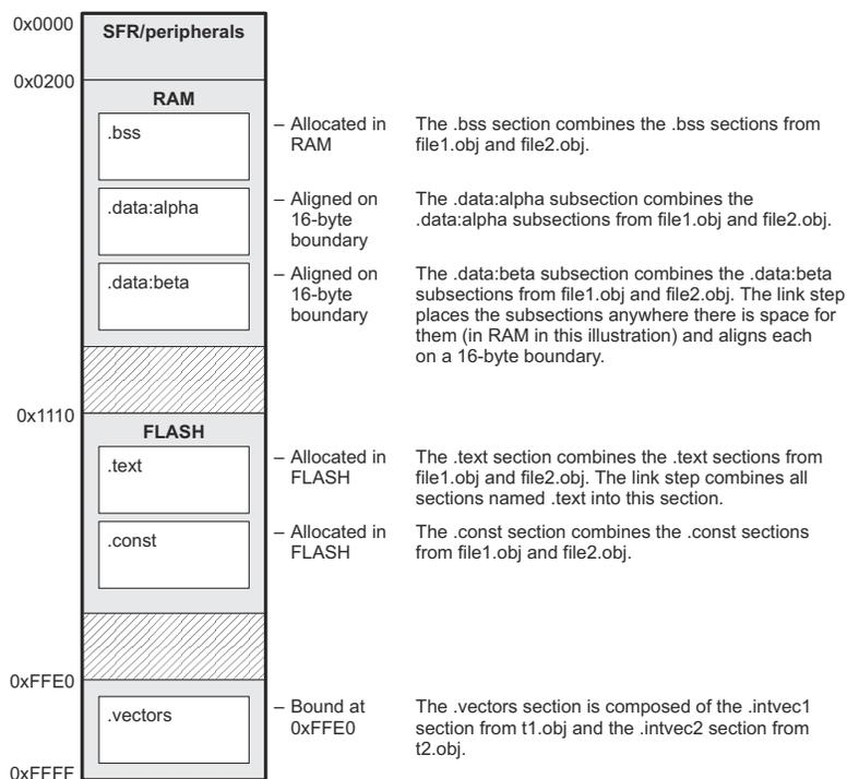
**Figure 8-2. Section Placement Defined by The SECTIONS Directive**
