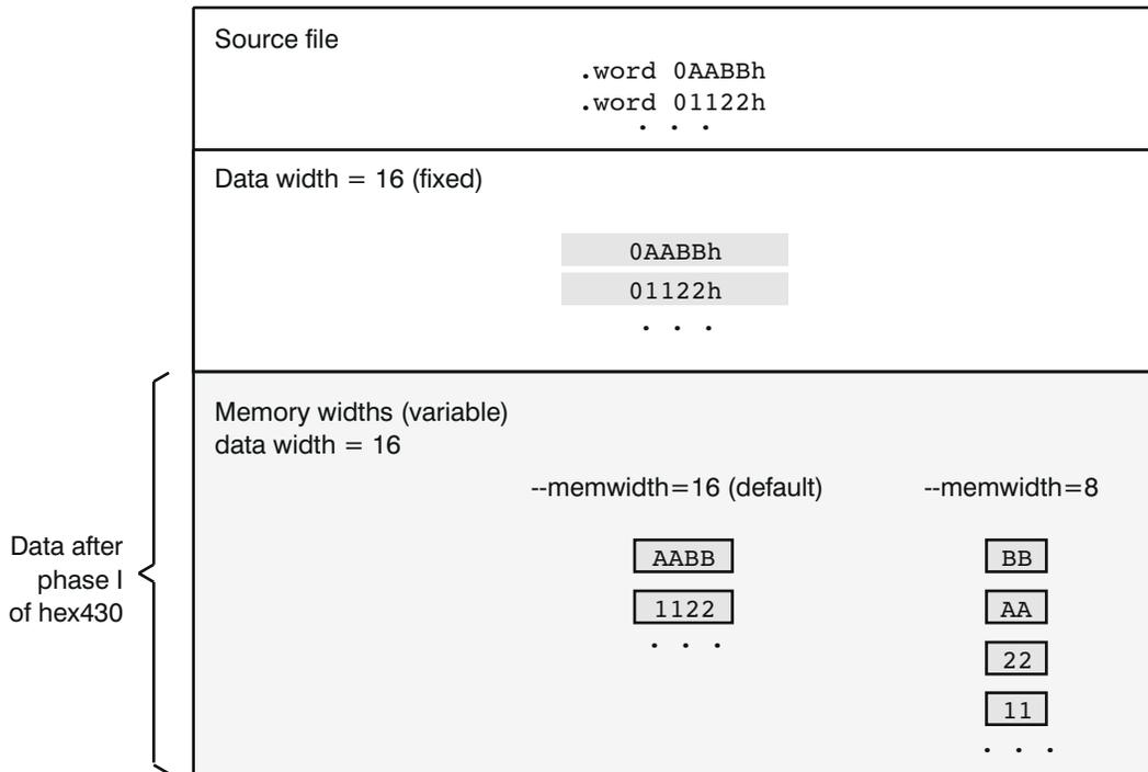
**Figure 12-3. Object File Data and Memory Widths**
