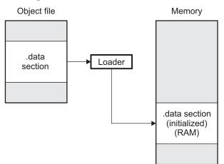
Figure 6-4. Initialization at Load Time
