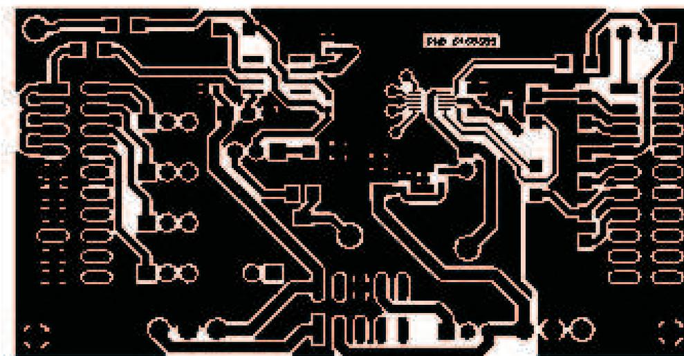
Figure 3. Top Layer (Signal and Split Ground Plane)
