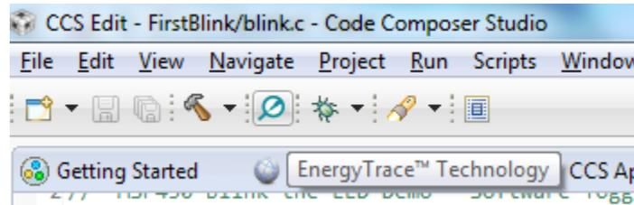
**Figure 4-2. EnergyTrace Button in the Toolbar Menu**
