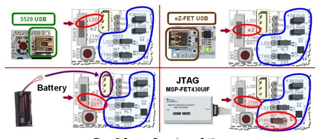
Figure 7. Common Power Jumper Settings
