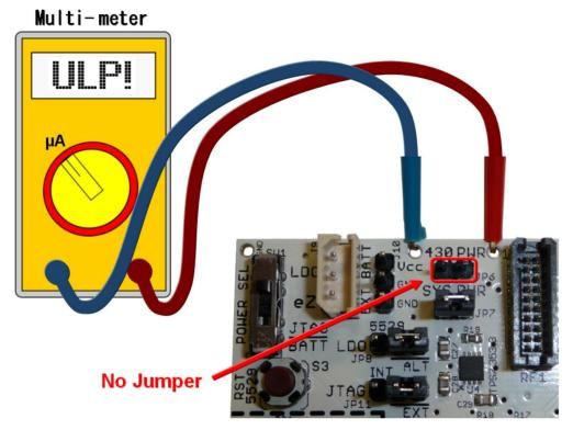
Figure 9. MSP430 Current Measurement Connection
