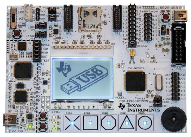
Figure 1. MSP-EXP430F5529 Experimenter's Board
