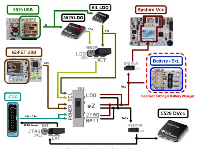
Figure 8. Visual Power Schematic
