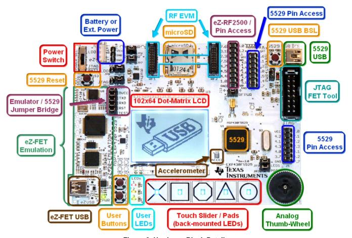
Figure 6. Hardware Block Details
