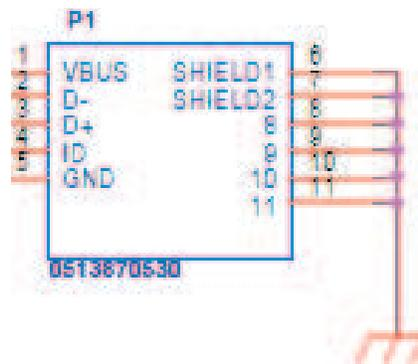
Figure 47. USB Mini Connector Pin Outs
