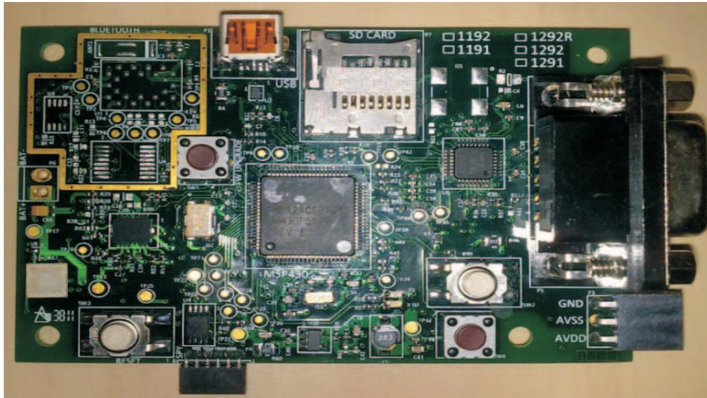
**Figure 1. ADS1x9x ECG-FE Demonstration Kit**
