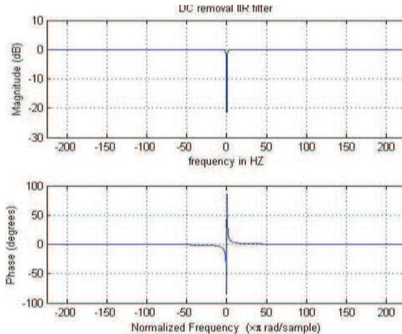
**Figure 38. Frequency Response for the IIR Filter**
